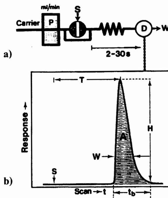
**Figure 2.12** a) The simplest single line FIA manifold utilizing a carrier stream of reagent;  $S$  is the injection port,  $D$  is the flow cell, and  $W$  is the waste. b). The analog output has the form of a peak, the recording starting at  $S$  (time of injection to).  $H$  is the peak height,  $W$  is the peak width at a selected level, and  $A$  is the peak area.  $T$  is the residence time corresponding to the peak height measurement, and  $t_b$  is the peak width at the baseline [56].
