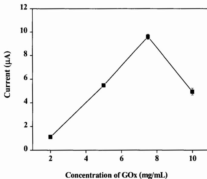
**Figure 4.4** The effect of GOx concentration (mg/ mL) on the current response obtained from 10 mM glucose in phosphate buffer solution (0.1 M, pH 7.0).
