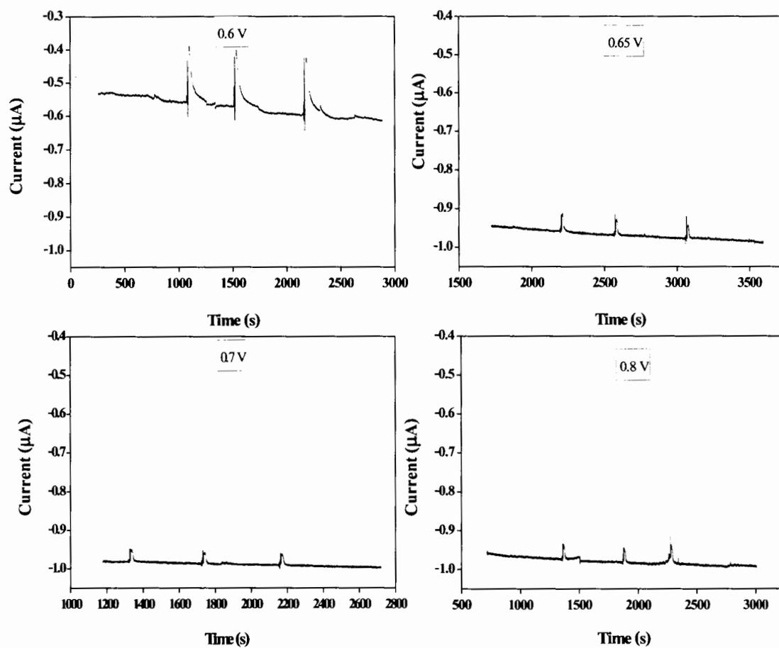
**Figure B.4** FIA gram of the applied potential on the GC/CNTs-NH<sub>2</sub>-Fc-BSA-GOx biosensor response 10 mM glucose, flow rate 1 mL/min (Continued).
