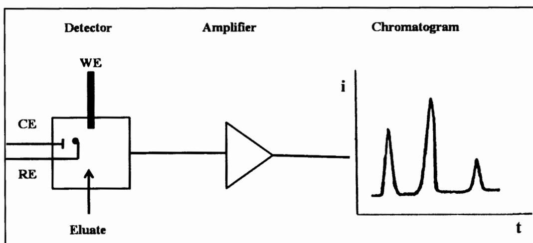
**Figure 2.10** Outline of amperometric detection. WE - working electrode; CE - counter electrode; RE - reference electrode. Adopted from [50].
