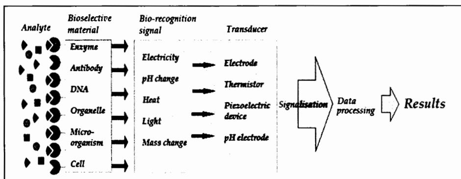
**Figure 2.1** Schematic of biosensor components (bioreceptor and transducer) [26].
