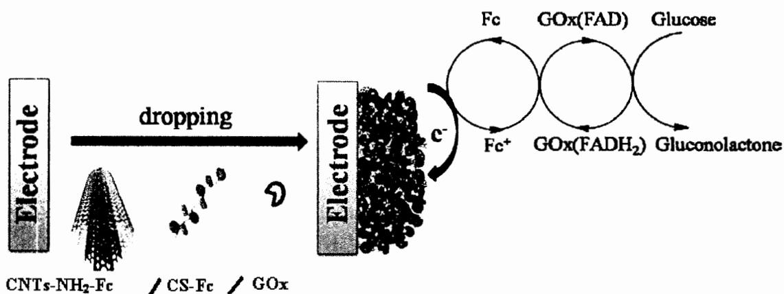
**Scheme 4.1** Schematic representation of the CNTs-NH<sub>2</sub>-Fc/CS-Fc/GOx modified electrode and the mechanism of the oxidation of glucose catalyzed by GOx and mediated by Fc.
