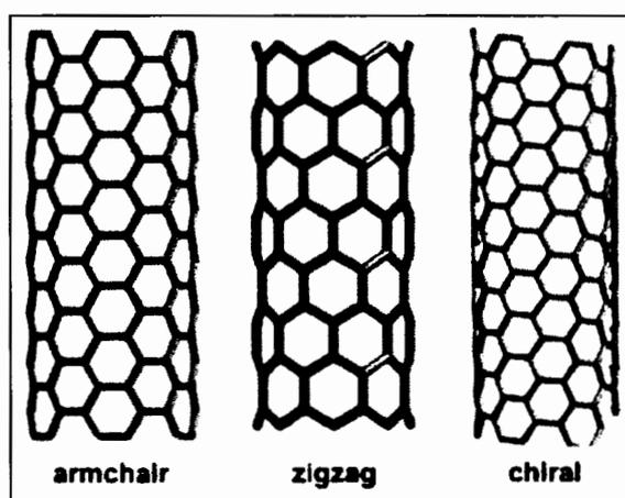
**Figure 2.5** SWCNTs with different chiralities. The difference in structure is easily shown at the open end of the tubes (armchair, zigzag s and chiral structure).
