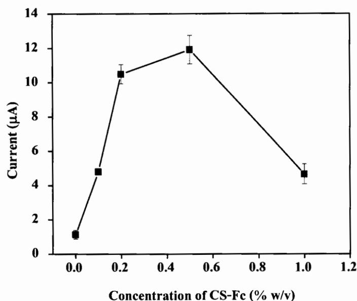
**Figure 4.3** The effect of concentration of CS-Fc (% w/v) on the oxidation current of 10 mM glucose solution in phosphate buffer solution pH 7.0.
