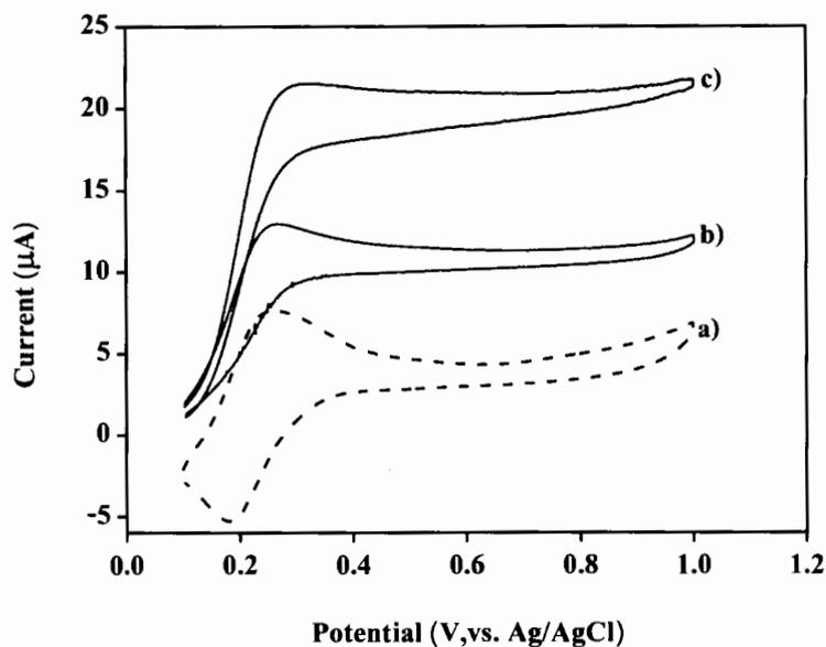
**Figure 4.6** Cyclic voltammograms obtained from the glucose biosensor (GC/CNTs-NH<sub>2</sub>-Fc/CS-Fc/GOx) in a) 0.1 M phosphate buffer b) 10 and c) 20 mM glucose.
