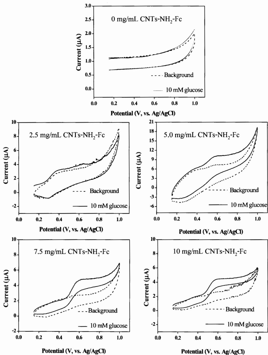
**Figure B.1** Cyclic voltammetric responses of 10 mM glucose on CNTs-NH<sub>2</sub>-Fc concentration in modified in electrode.
