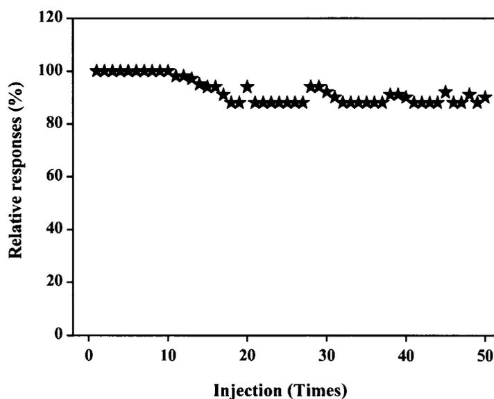
**Figure 4.23** Operational stability of the CNTs-NH<sub>2</sub>-Fc-BSA-GOx glucose biosensor to repeated injections of 10 mM glucose.
