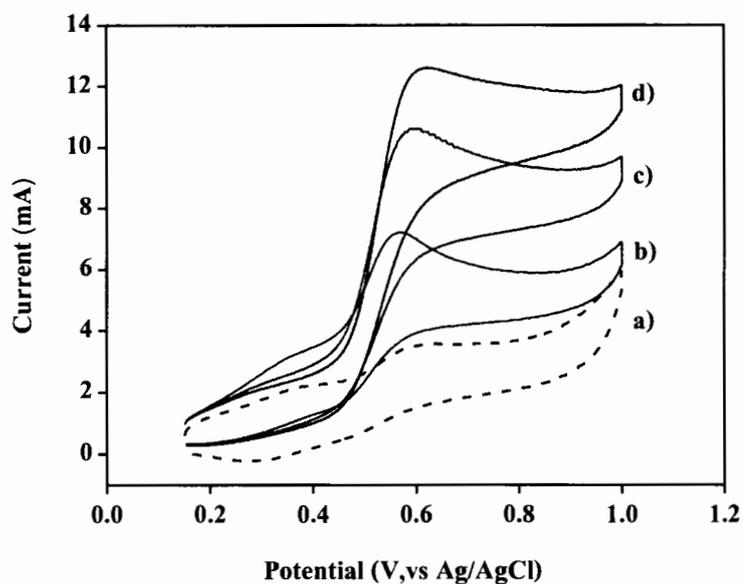
**Figure 4.17** Cyclic voltammograms of the glucose biosensor (GC/CNTs- $\text{NH}_2$ -Fc-BSA-GOx) a) 0.1 M phosphate buffer, b) 5, c) 10 and d) 15 mM of glucose.
