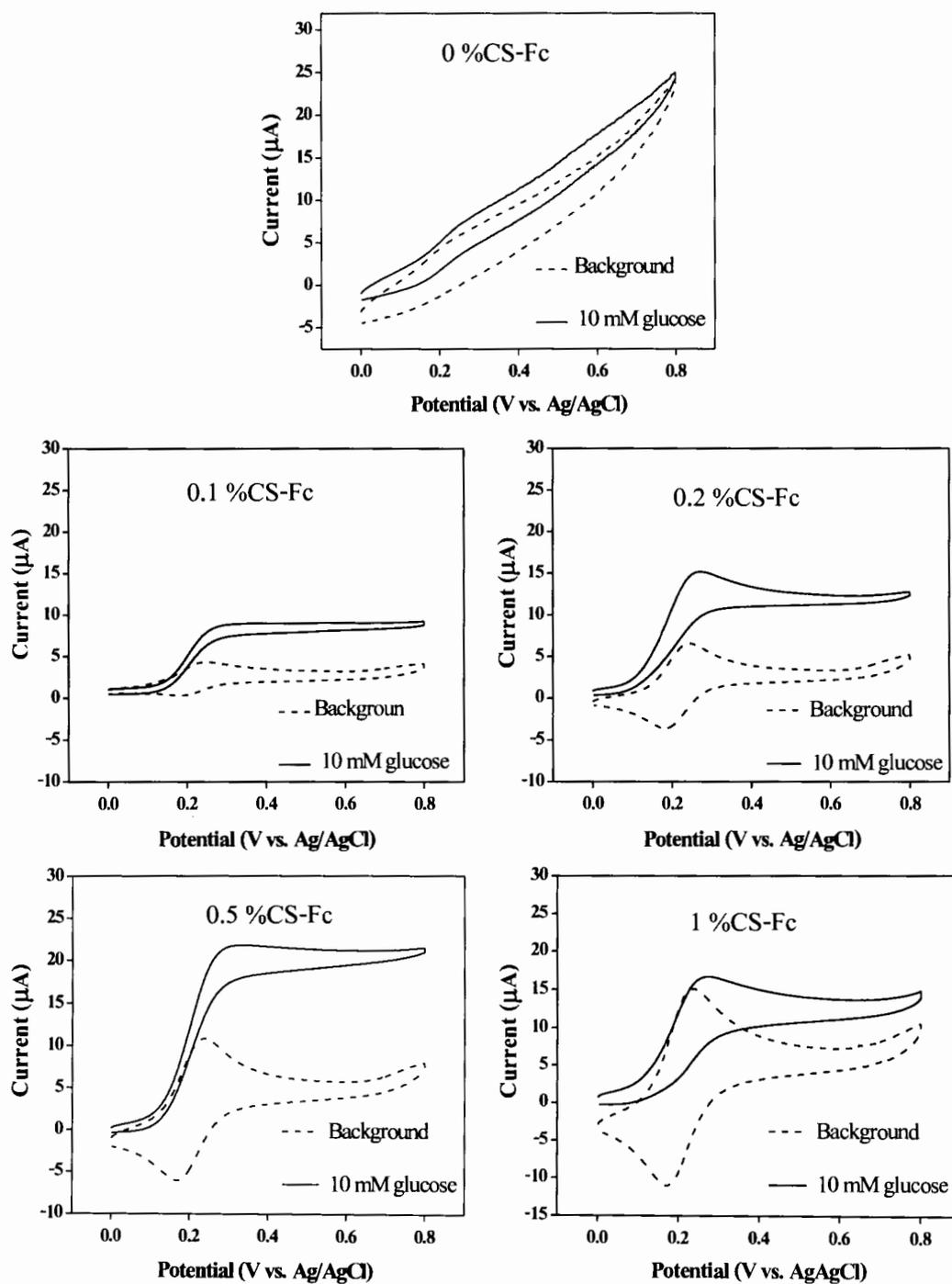
**Figure A.2** Cyclic voltammetric responses of 10 mM glucose CS-Fc concentration in modified electrode.
