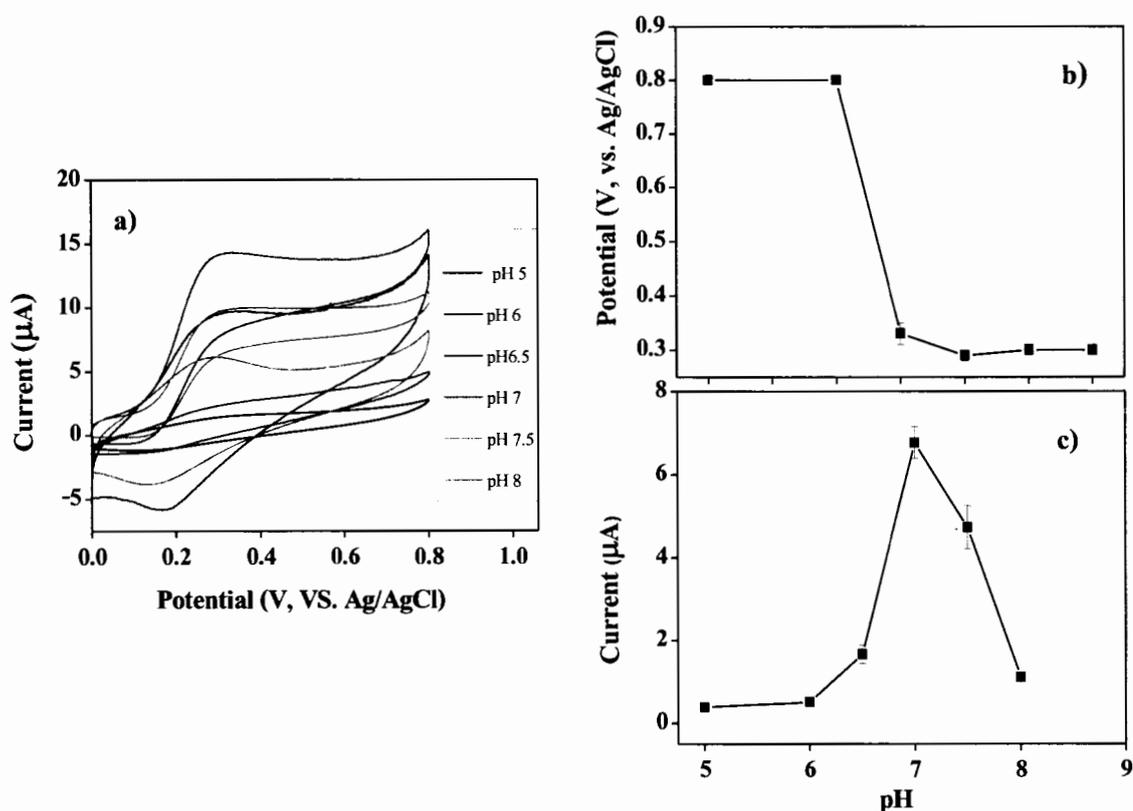
**Figure 4.5** a) Cyclic voltammetric responses of 10 mM glucose at various buffer pH and the dependence of buffer pH on b) peak potential, c) peak current obtained from the biosensor (GC/CNTs-NH<sub>2</sub>-Fc/CS-Fc/GOx).
