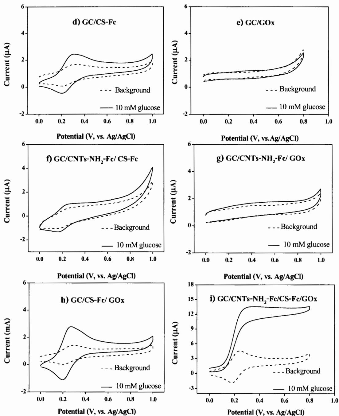
**Figure 4.1** Cyclic voltammograms of a) bare glassy carbon electrode (GC) in the absence (dotted line) and presence of 10 mM glucose (solid line), b) GC/CNTs-NH<sub>2</sub>-Fc, c) GC/CS, d) GC/CS-Fc, (e) GC/GOx, f) GC/CNTs-NH<sub>2</sub>-Fc/CS-Fc, g) GC/CNTs-NH<sub>2</sub>-Fc/GOx, h) GC/CS-Fc/GOx, and i) GC/CNTs-NH<sub>2</sub>-Fc/CS-Fc/GOx in 0.1 M phosphate buffer pH 7.0 (Continued).
