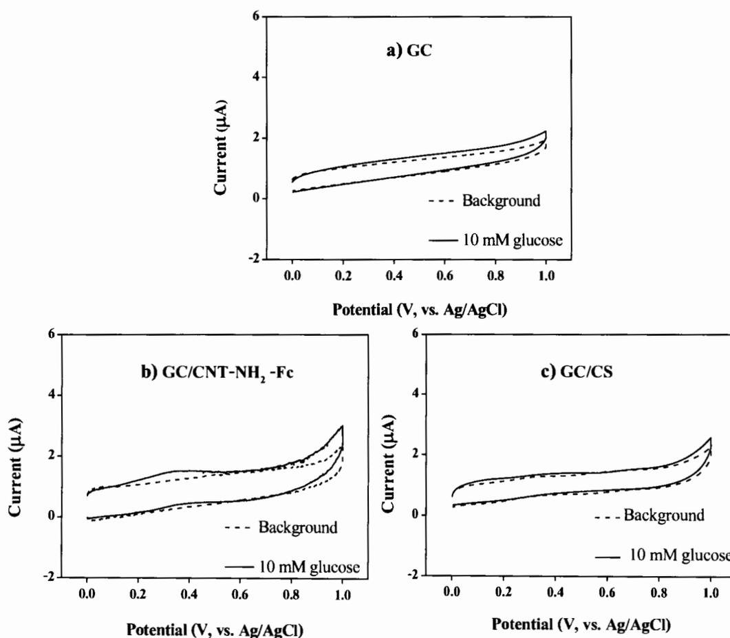
**Figure 4.1** Cyclic voltammograms of a) bare glassy carbon electrode (GC) in the absence (dotted line) and presence (solid line) of 10 mM glucose, b) GC/CNTs-NH<sub>2</sub>-Fc, c) GC/CS, d) GC/CS-Fc, e) GC/GOx, f) GC/CNTs-NH<sub>2</sub>-Fc/CS-Fc, g) GC/CNTs-NH<sub>2</sub>-Fc/GOx, h) GC/CS-Fc/GOx, and i) GC/CNTs-NH<sub>2</sub>-Fc/CS-Fc/GOx in 0.1 M phosphate buffer pH 7.0.
