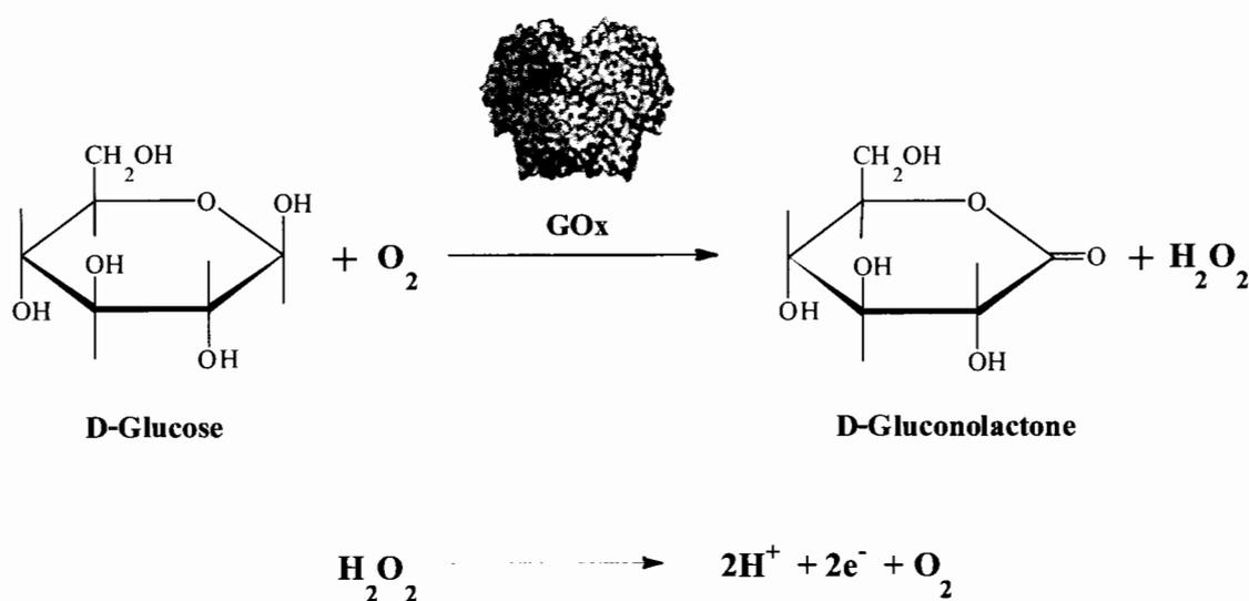
**Figure 2.4** Schematic diagram of glucose oxidase (GOx) enzymatic reaction [36].
