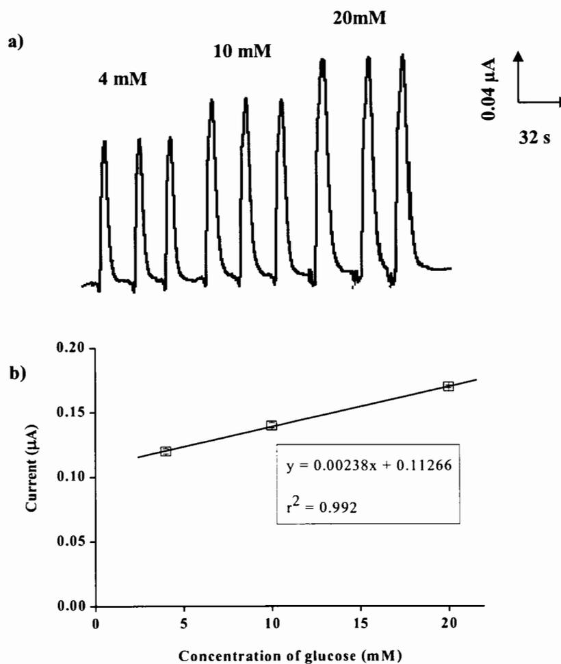
**Figure 4.22** Response to standard glucose a) and the corresponding standard glucose calibration curve b). Flow rate 1.0 mL/min, applied potential 0.6 V.
