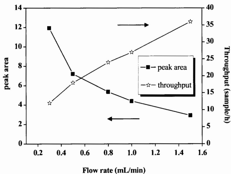
**Figure 4.19** Effect of the flow rate on glucose biosensor response and sample throughput.
