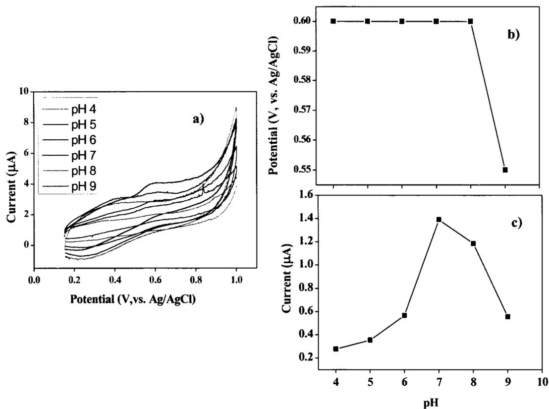
**Figure 4.16** a) Cyclic voltammetric responses of 10 mM glucose at various buffer pH and the dependence of buffer pH on the b) peak potential, c) peak current obtained from the biosensor.
