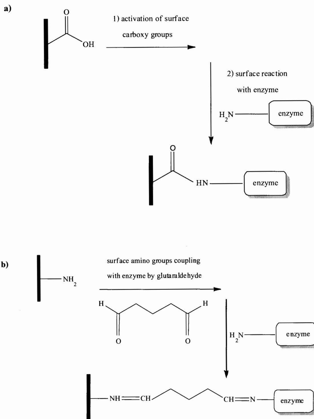
**Figure 2.3** Examples of covalent linkage of enzyme layers to solid surfaces by coupling of a) carboxy and b) amino functionalities [35].
