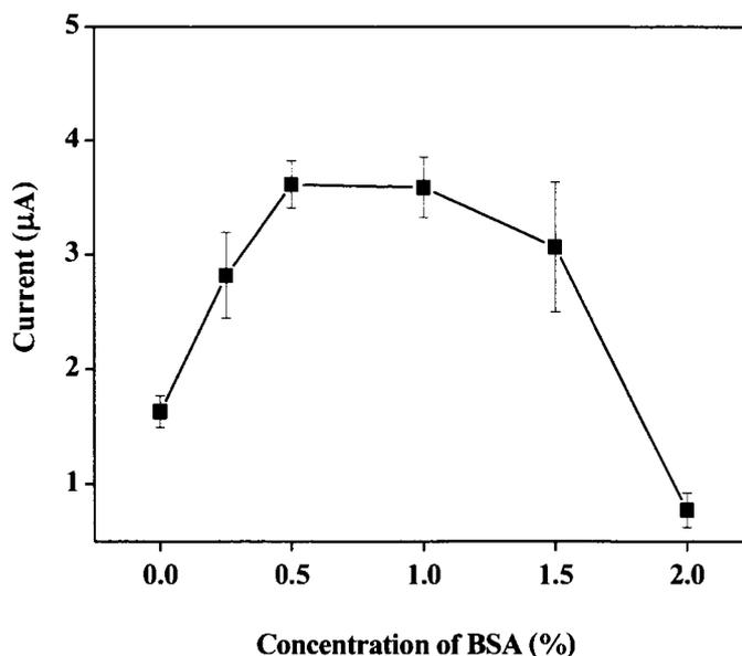
**Figure 4.14** The effect of the concentration of BSA (%) on the cyclic voltametry response of oxidation current to 10 mM glucose solution in phosphate buffer solution pH 7.0
