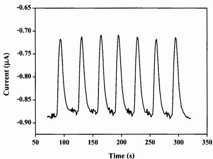
**Figure 4.21** FI amperometric response obtained from the developed sulfite biosensor for 7 repetitive injection of 2 mM glucose. Carrier solution; 0.1 M phosphate buffer pH 7.0, applied potential 0.6 V, flow rate; 1.0 mL/min.
