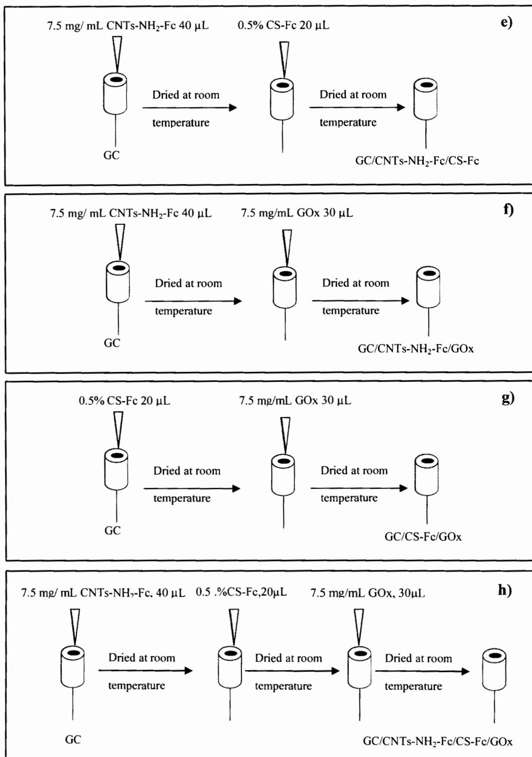
**Figure 3.2** Preparation procedure of a) GC/CNTs-NH<sub>2</sub>-Fc, b) GC/CS, c) GC/CS-Fc, d) GC/GOx, e) GC/CNTs-NH<sub>2</sub>-Fc/CS-Fc, f) GC/CNTs-NH<sub>2</sub>-Fc/GOx, g) GC/CS-Fc/GOx and h) GC/CNTs-NH<sub>2</sub>-Fc/CS-Fc/GOx electrode (Continued).
