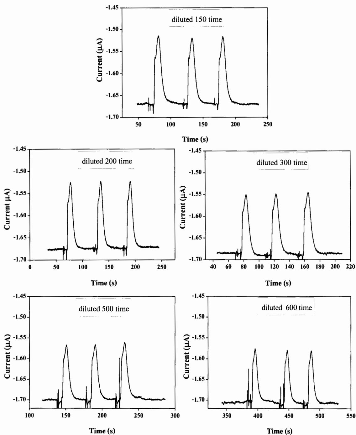
**Figure B.7** FIA gram of the sample on the GC/CNTs-NH<sub>2</sub>-Fc-BSA-GOx biosensor at 0.6 V, flow rate 1 mL/min.
