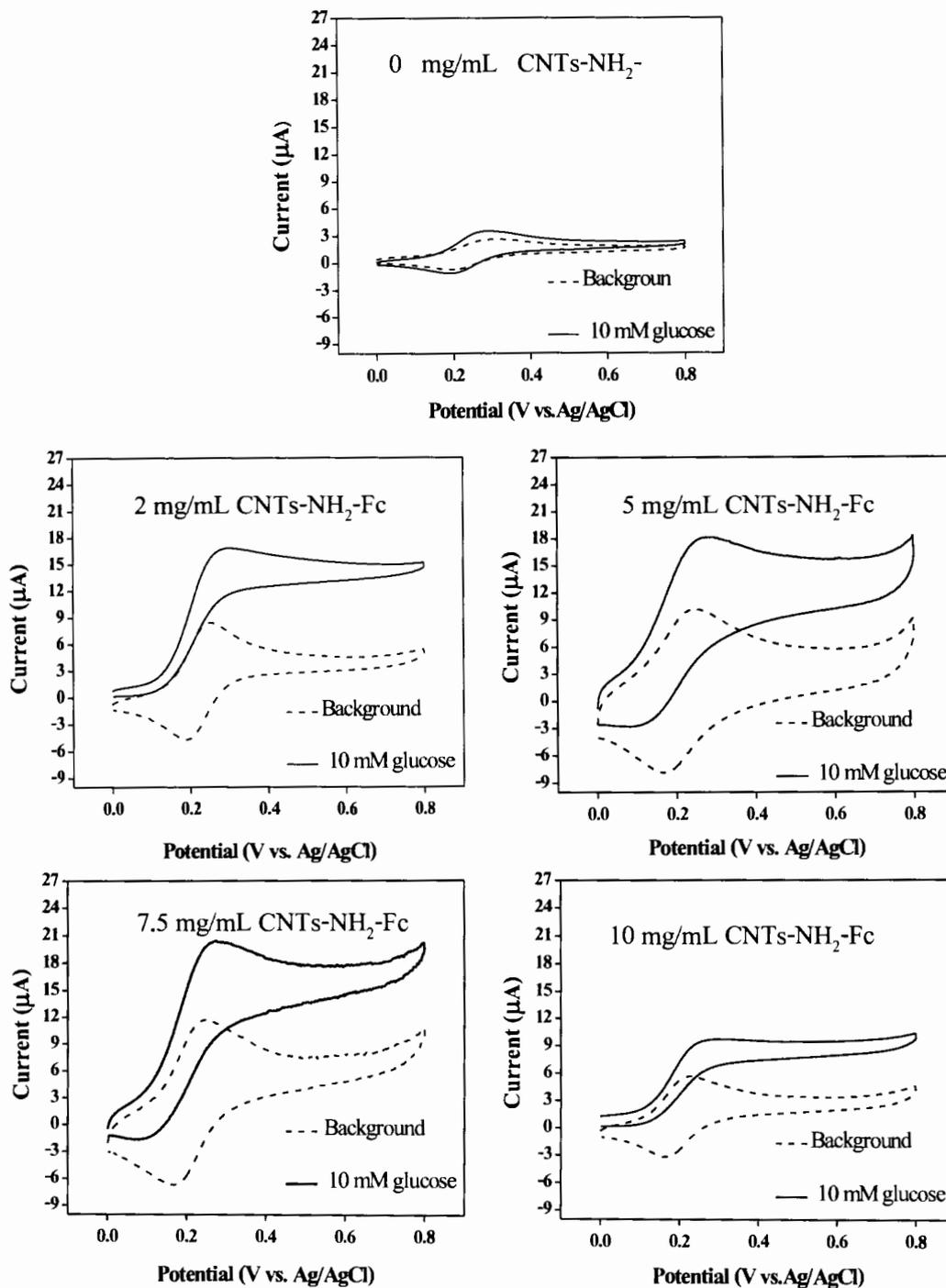
Figure A.1 Cyclicvoltammetric responses of 10 mM glucose at various concentration of CNTs-NH<sub>2</sub>-Fc (mg/mL).
