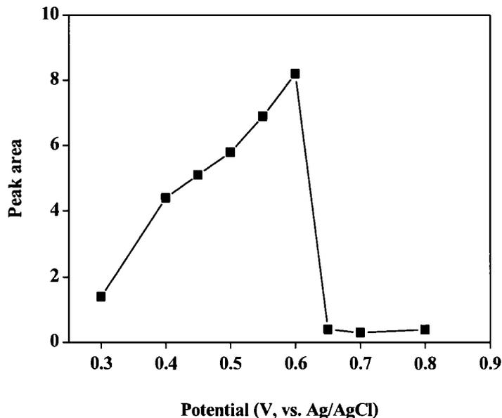
**Figure 4.18** Effect of operating potential on the biosensor response studied by amperometric measurement of 10 mM glucose in 0.1M phosphate buffer (pH 7.0).
