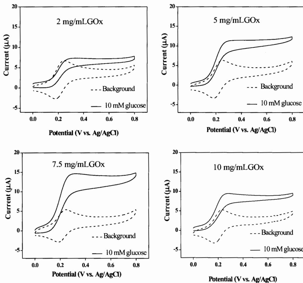
**Figure A.3** Cyclic voltammetric responses of 10 mM glucose on GOx concentration in modified in electrode.
