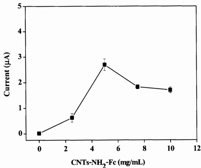
**Figure 4.13** The effect of the concentration of CNTs-NH<sub>2</sub>-Fc (mg/ mL) on the cyclic voltametry response of oxidation current to 10 mM glucose solution in phosphate buffer solution pH 7.0 .
