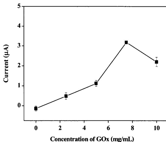
**Figure 4.15** The effect of the concentration of GOx (mg/ mL) on the cyclic voltametry response of oxidation current to 10 mM glucose solution in phosphate buffer solution pH 7.0.
