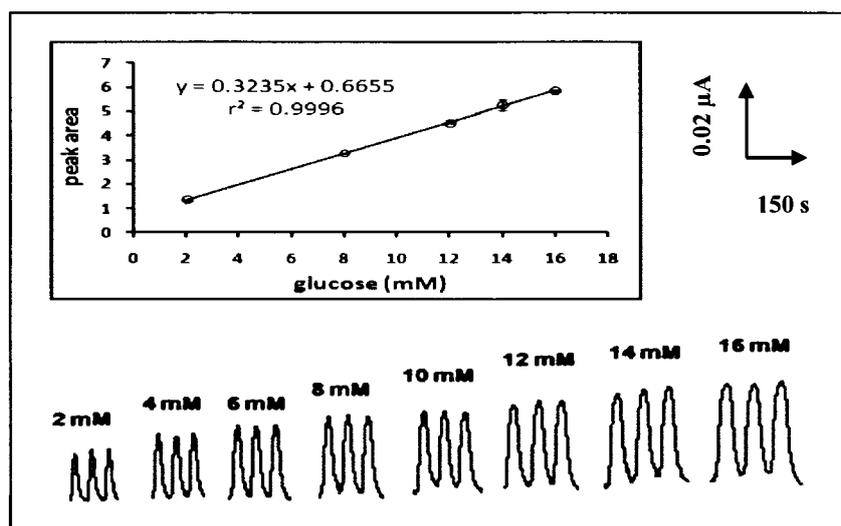
**Figure 4.20** FIA diagram of injected glucose concentration within 2 - 16 mM in to phosphate buffer solution pH 7.0, operating potential 0.6 V vs Ag/AgCl, flow rate 1 mL/min, injection volume of 20  $\mu$ L. The inset shows the linear relationship between the signal of glucose and the concentration.
