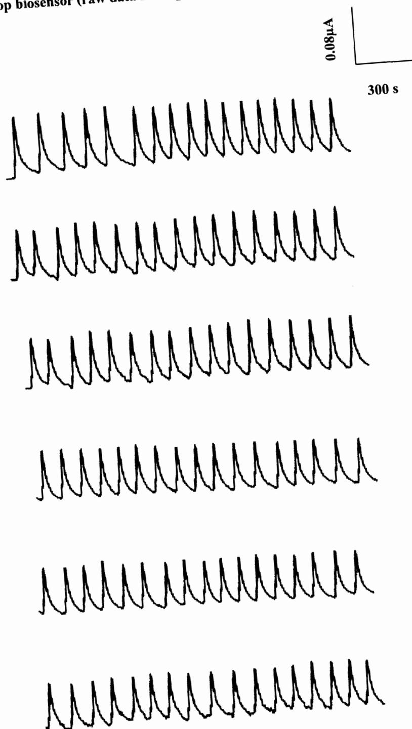
**Figure B.8** FIA gram of stability on the GC/CNTs-NH<sub>2</sub>-Fc-BSA-GOx biosensor.
