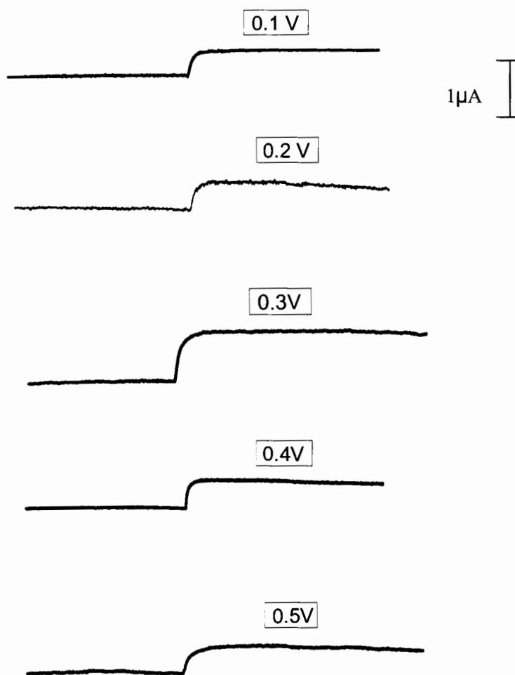
**Figure A.4** Amperogram of the applied potential on the GC/CNTs-NH<sub>2</sub>-Fc/CS-Fc/GOx biosensor response 0.5 mM glucose.
