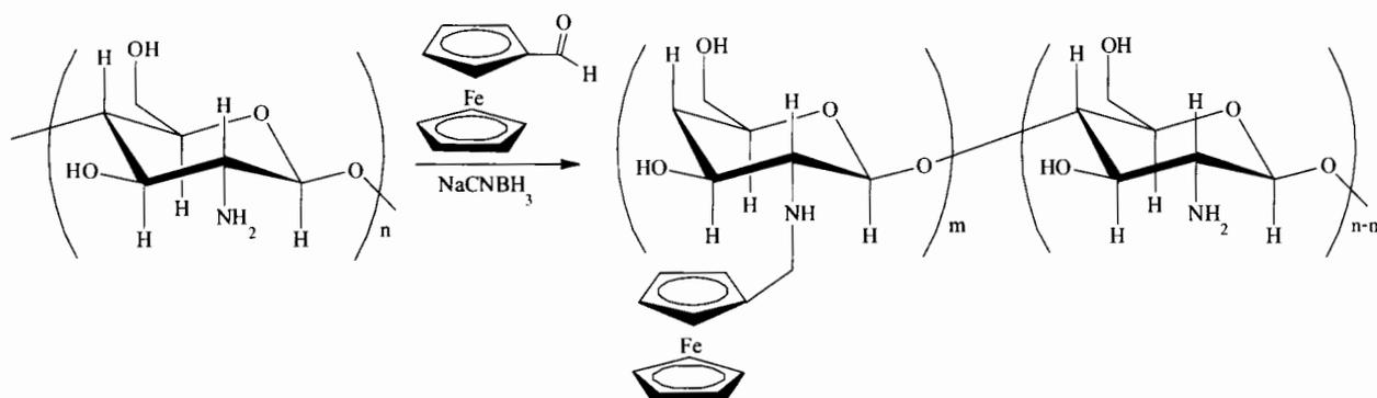
**Figure 3.1** Synthesis of ferrocene bound chitosan (CS-Fc).
