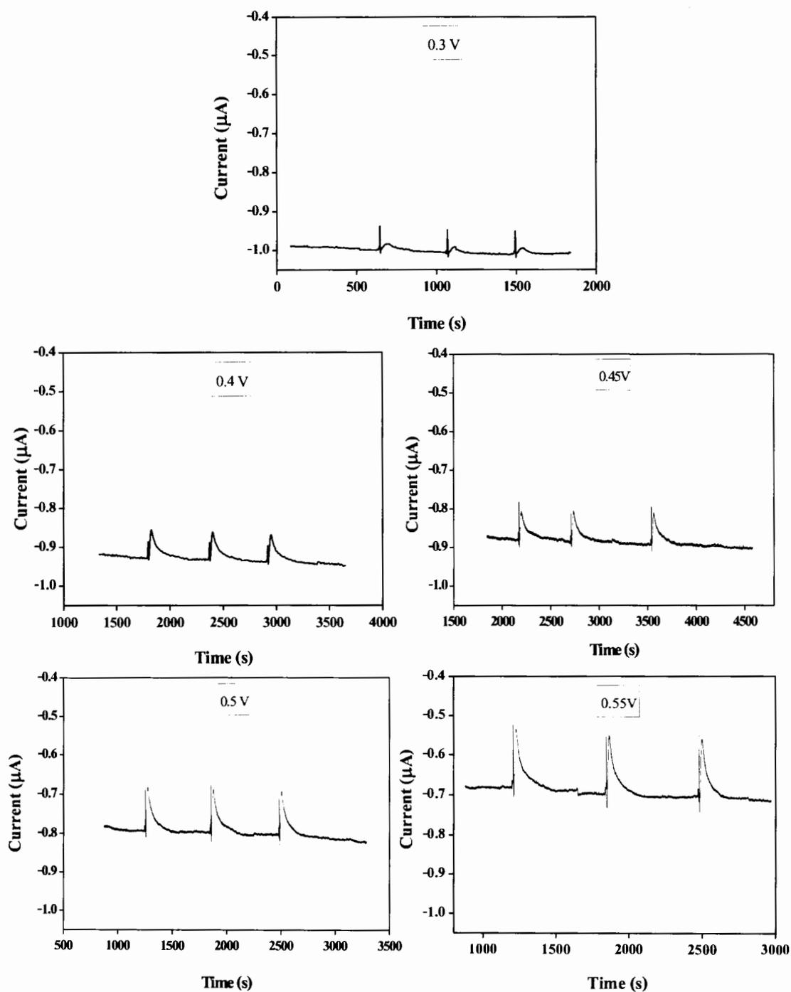
**Figure B.4** FIA gram of the applied potential on the GC/CNTs-NH<sub>2</sub>-Fc-BSA-GOx biosensor response 10 mM glucose, flow rate 1 mL/min.
