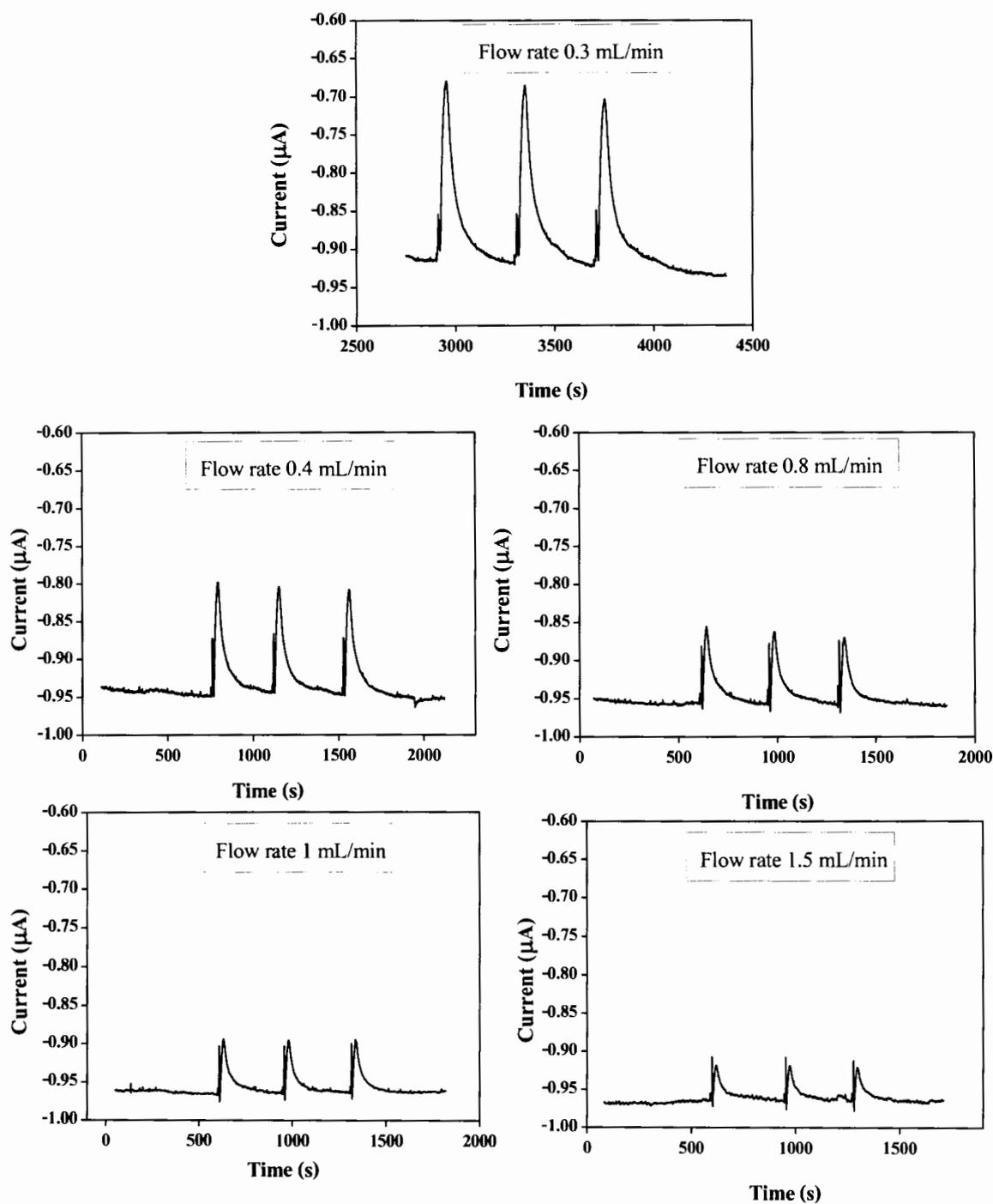
**Figure B.5** FIA gram of flow rate on the GC/CNTs-NH<sub>2</sub>-Fc-BSA-GOx biosensor response 10 mM glucose, applied potential at 0.6 V.
