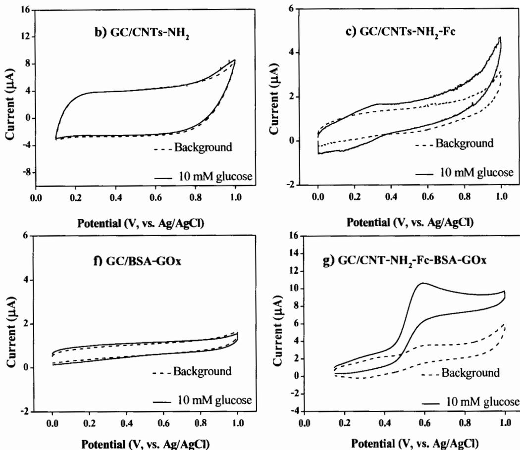
**Figure 4.12** Cyclic voltammograms for a) bare glassy carbon electrode (GC) in the absent (dotted line) and present of 10 mM glucose (solid line), b) GC/CNTs-NH<sub>2</sub>, c) GC/CNTs-NH<sub>2</sub>-Fc, d) BSA, e) GC/GOx, f) GC/BSA-GOx and g) GC/CNTs-NH<sub>2</sub>-Fc-BSA-GOx in 0.1 M phosphate buffer pH 7.0 (Continued).
