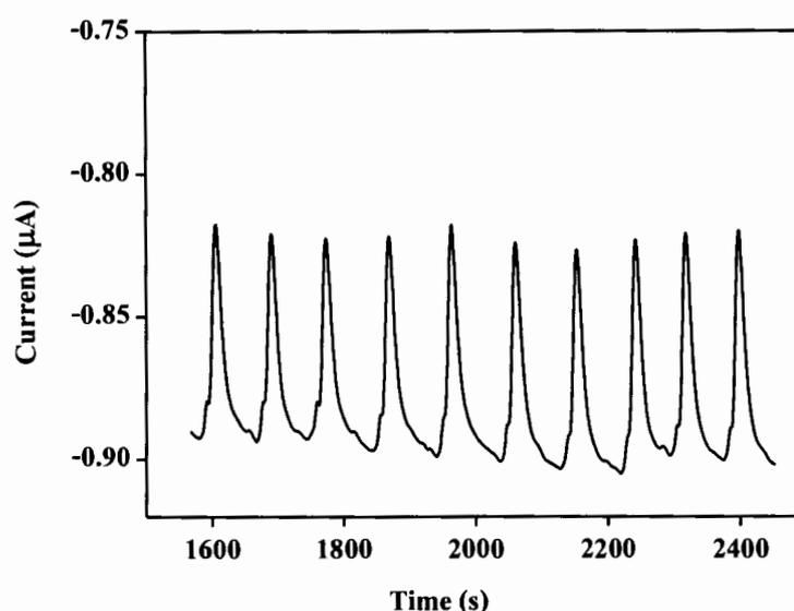
**Figure 4.9** An FI amperometric response obtained from the developed glucose biosensor for 10 repetitive injection of 10 mM glucose. Carrier solution; 0.1 M phosphate buffer pH 7.0, applied potential; 0.3 V, flow rate; 1.0 mL/min.
