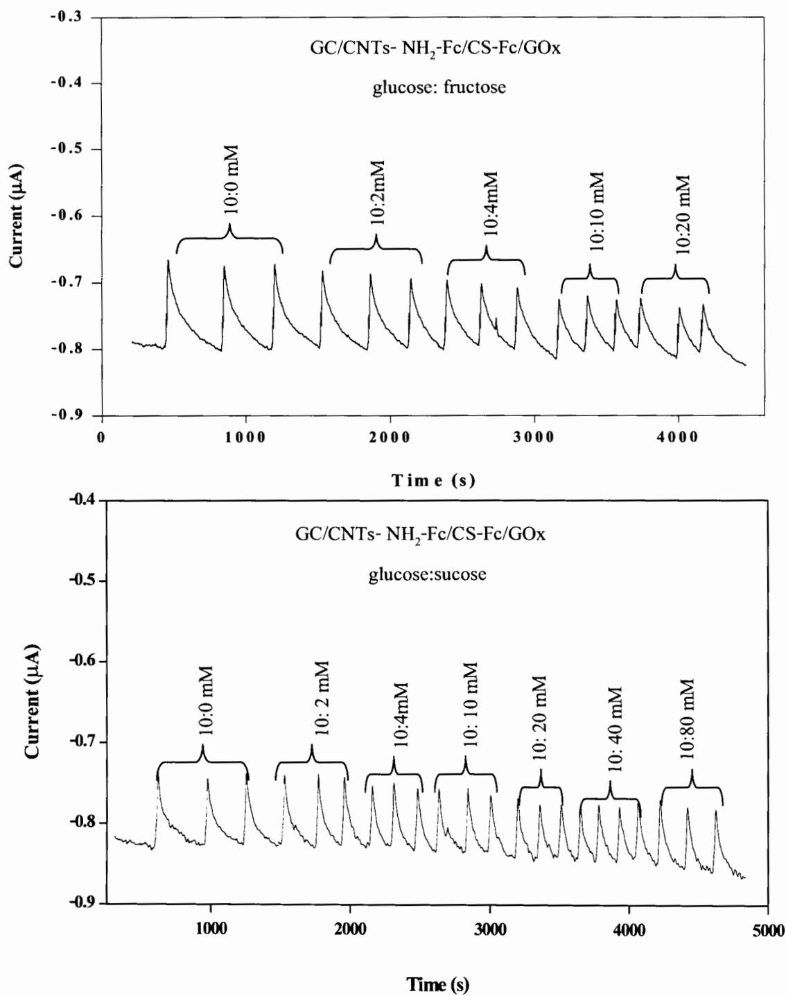
**Figure A.5** FIA gram of the interference on the GC/CNTs-NH<sub>2</sub>-Fc/CS-Fc/GOx biosensor
