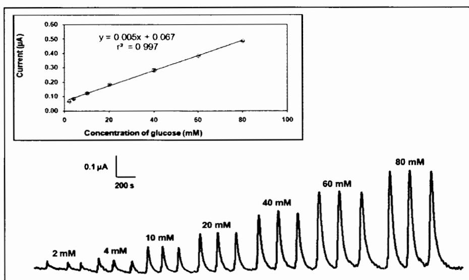
**Figure 4.8** An FIA diagram of injected glucose concentration within 2 - 80 mM into phosphate buffer solution pH 7.0, operating potential 0.3 V vs Ag/AgCl, flow rate 1 mL/min, injection volume of 20 μL. The inset shows the linear relationship between the signal of glucose and the concentration.
