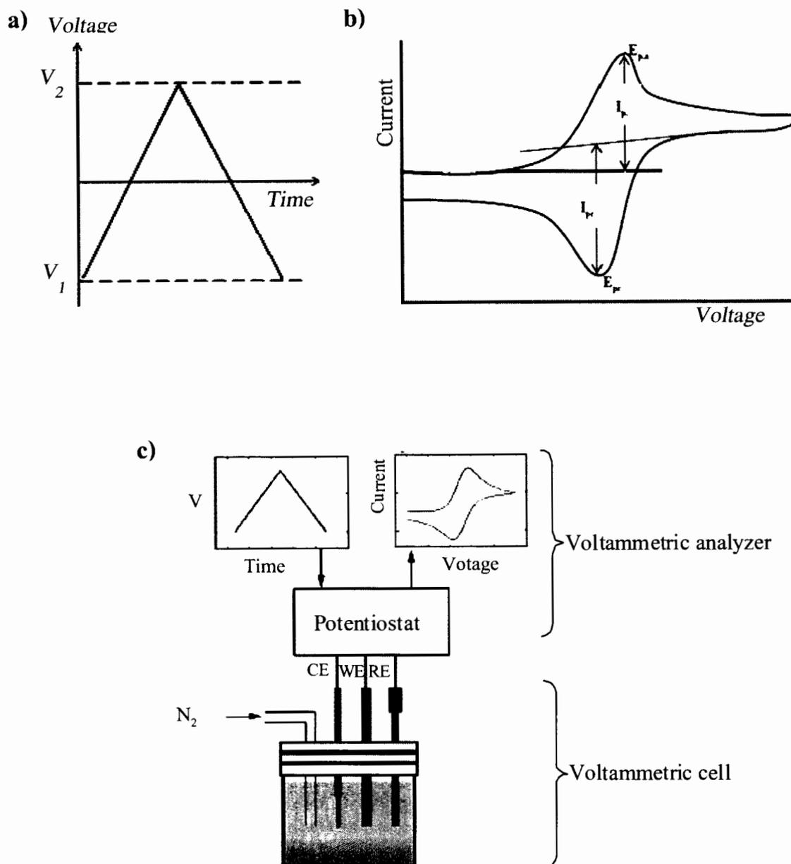
**Figure 2.11** Typical of a) cyclic voltammogram wave from: variation of the potential applied to the working electrode with time, b) cyclic votammogram: resulting current-potential curves, c) voltammetric or components of cyclic voltammetry systems which composed of voltammetric analyzer and voltammetric cell adopted from [53].
