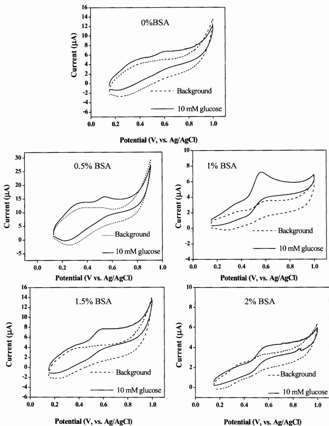
**Figure B.2** Cyclic voltammetric responses of 10 mM glucose on BSA concentration in modified in electrode.
