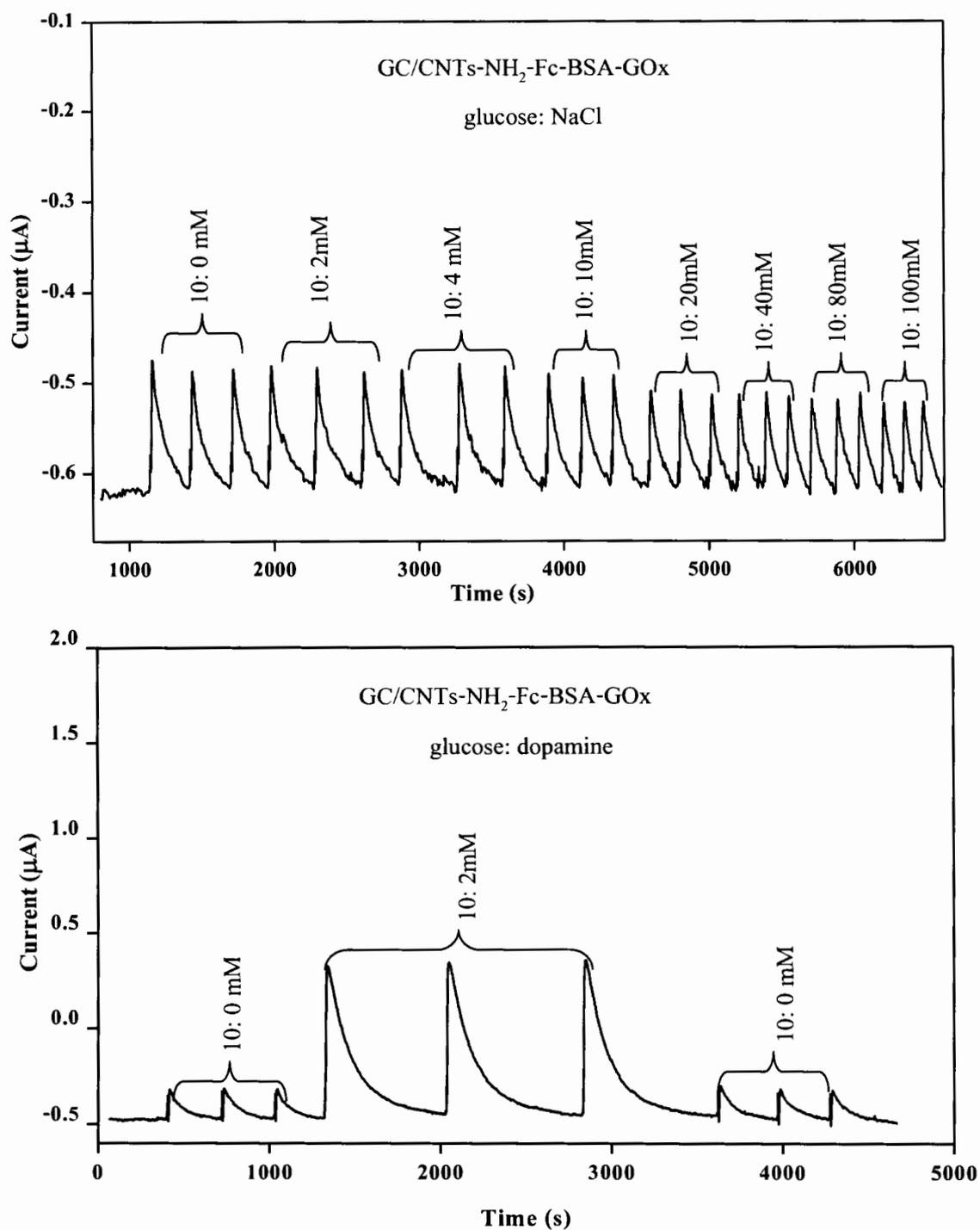
**Figure B 6** FIA gram of the interference on the GC/CNTs-NH<sub>2</sub>-Fc-BSA-GOx biosensor at 0.6 V, flow rate 1 mL/min (Continued).
