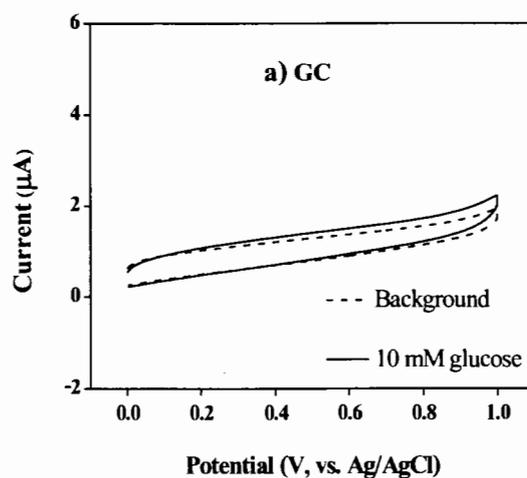
**Figure 4.12** Cyclic voltammograms for a) bare glassy carbon electrode (GC) in the absent (dotted line) and present of 10 mM glucose (solid line), b) GC/CNTs-NH<sub>2</sub>, c) GC/CNTs-NH<sub>2</sub>-Fc, d) BSA, e) GC/GOx, f) GC/BSA-GOx and g) GC/CNTs-NH<sub>2</sub>-Fc-BSA-GOx in 0.1 M phosphate buffer pH 7.0.
