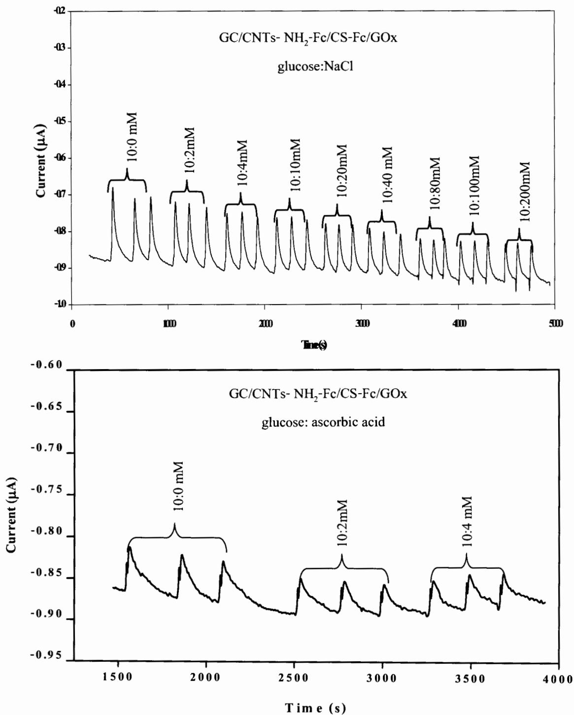
Figure A.5 FIA gram of the interference on the GC/CNTs- $\text{NH}_2\text{-Fc/CS-Fc/GOx}$  biosensor.
