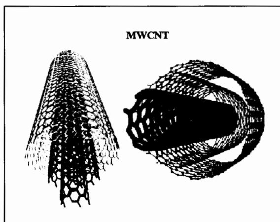
**Figure 2.6** Structure of multi-walled carbon nanotubes (MWCNTs).
