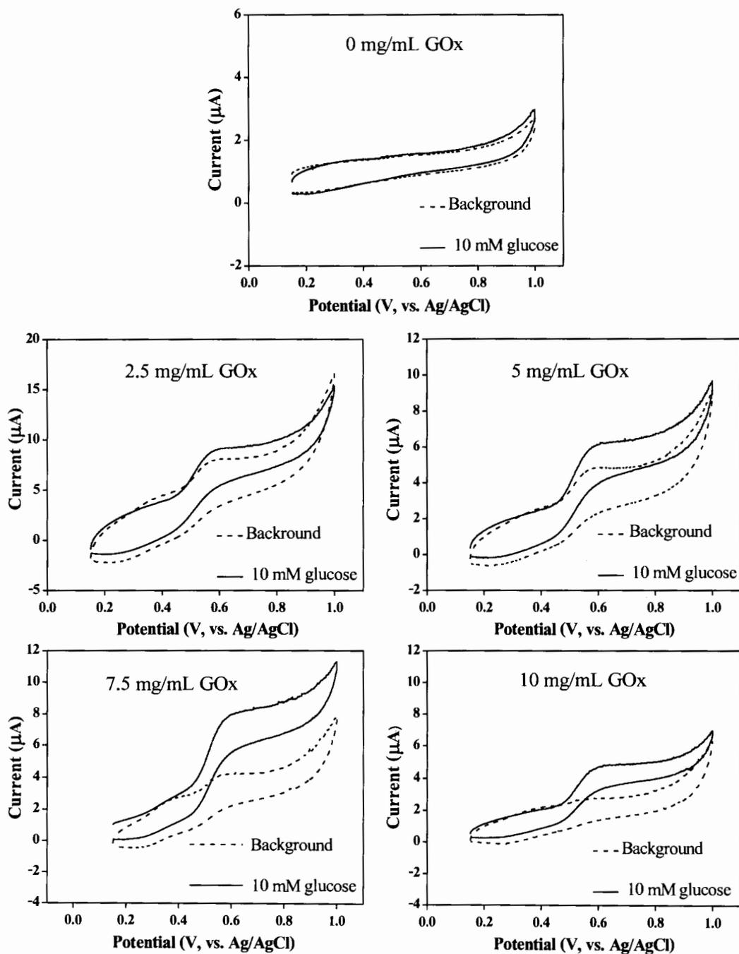
**Figure B.3** Cyclic voltammetric responses of 10 mM glucose on glucose oxidase (GOx) concentration in modified in electrode.
