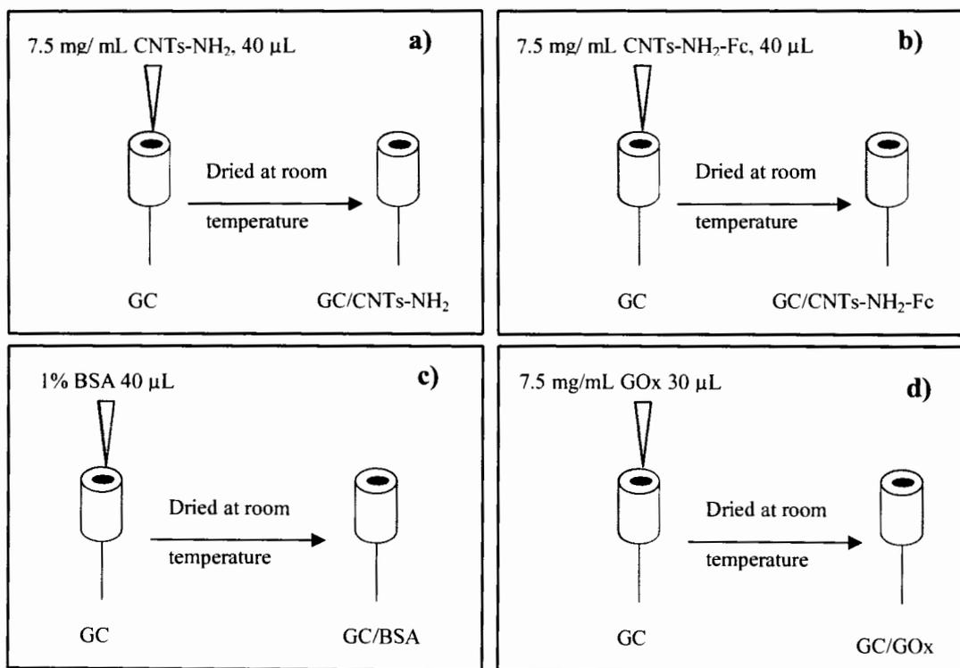
**Figure 3.5** Preparation procedure of a) GC/CNTs-NH<sub>2</sub> b) GC/CNTs-NH<sub>2</sub>-Fc, c) GC/BSA, d) GC/GOx, e) GC/BSA-GOx and f) GC/CNTs-NH<sub>2</sub>-Fc-BSA-GOx electrodes.
