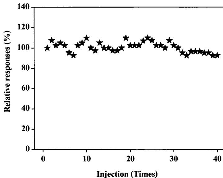
**Figure 4.10** Operational stability of the CNTs-NH<sub>2</sub>-Fc/CS-Fc/GOx glucose biosensor to repeatedly injections of 10 mM glucose.
