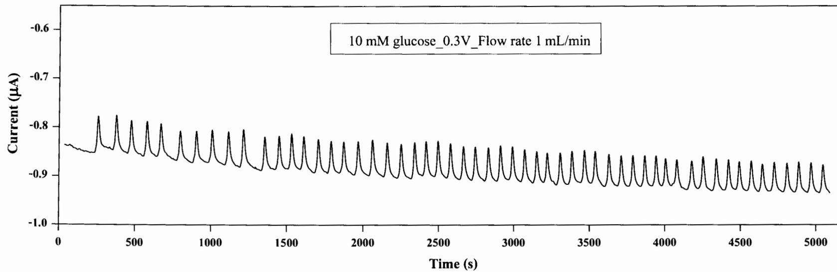
Figure A.6 FIA gram of stability on the GC/CNTs-NH<sub>2</sub>-Fc/CS-Fc/GOx biosensor.
