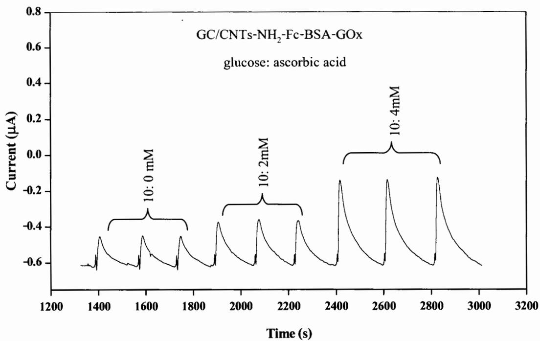
**Figure B 6** FIA gram of the interference on the GC/CNTs-NH<sub>2</sub>-Fc-BSA-GOx biosensor at 0.6 V, flow rate 1 mL/min (Continued).
