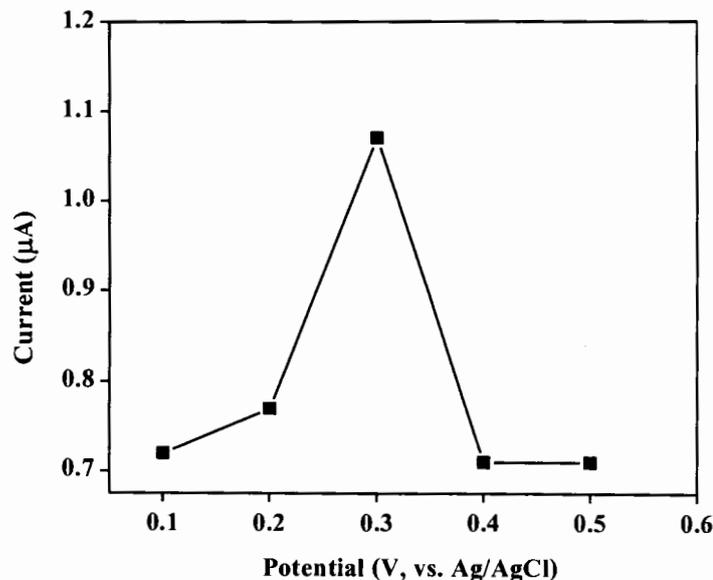
**Figure 4.7** Effect of the applied potential on glucose detection using the GC/CNTs-NH<sub>2</sub>-Fc/CS-Fc/GOx electrode. The current obtained from 0.5 mM glucose in phosphate buffer (0.1 M, pH 7.0).
