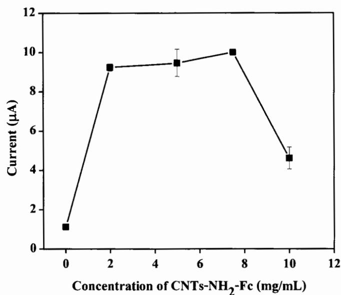
**Figure 4.2** The effect of the concentration of CNTs-NH<sub>2</sub>-Fc (mg/ mL) on oxidation current of 10 mM glucose solution in 0.1 M phosphate buffer solution pH 7.0.
