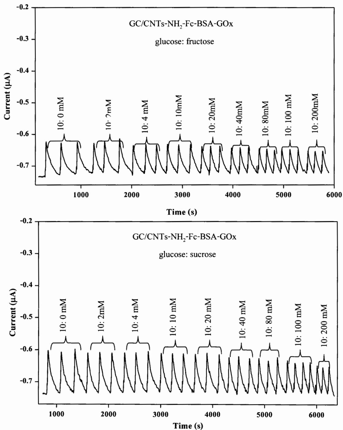
**Figure B 6** FIA gram of the interference on the GC/CNTs-NH<sub>2</sub>-Fc-BSA-GOx biosensor at 0.6 V, flow rate 1 mL/min.
