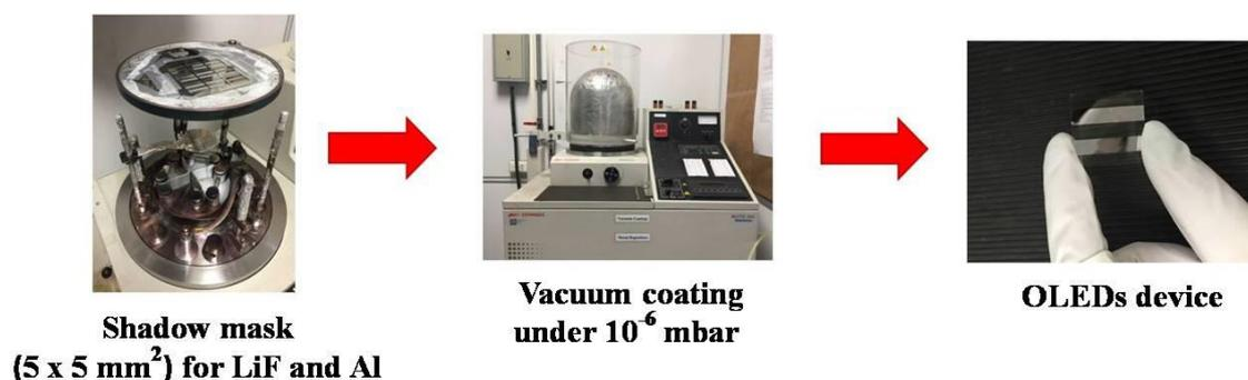
**Figure 3.3 Coating process of cathode electrode**
