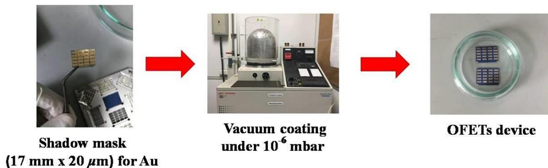
**Figure 3.6 Coating process of source-drain-gate electrodes**
