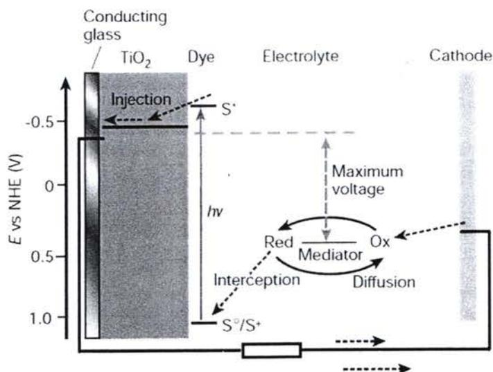
**Figure 2.2** The schematic operation of DSSCs [8].
