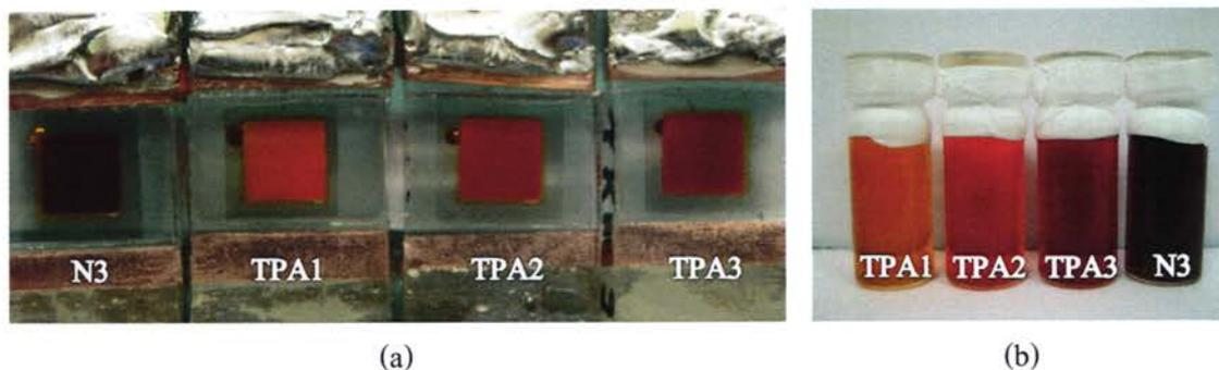
**Figure 4.8** The photograph of (a) DSSC devices and (b) dye solution based on TPA1-3 dye.
