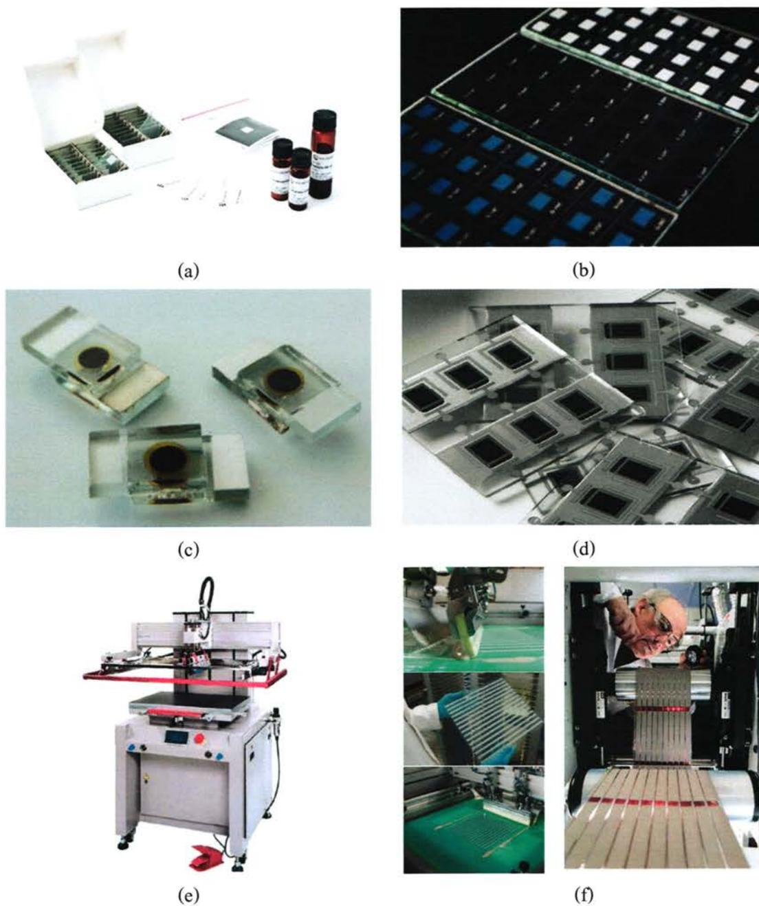
**Figure 2.15** A photograph of the DSSCs working electrode technology. (a) Soloronix education kits, (b) Dyesol pre-cut test-cell glass plate, (c) Soloronix spot cell kit, (d) ECN lab's homemade test cell, (e) semi-automate screen printer and (f) screen printing process and a piece of  $\text{TiO}_2$  green on conducting glass substrate [48-50].
