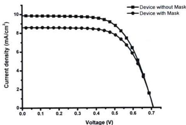
**Figure 4.5** The  $J$ - $V$  curves of DSSCs device measured with and without mask.
