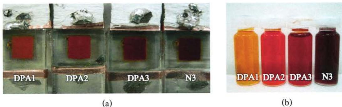
**Figure 4.11** The photograph of (a) DSSC devices and (b) dye solution based on DPA1-3 dye.
