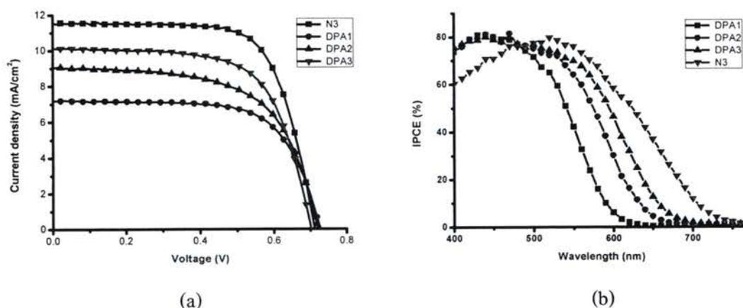
**Figure 4.12** (a) the  $J$ - $V$  characteristics (b) photocurrent action spectra of cells based on DPA1-3 sensitizer measured under irradiance of  $100 \text{ mW/cm}^2$  AM 1.5G.
