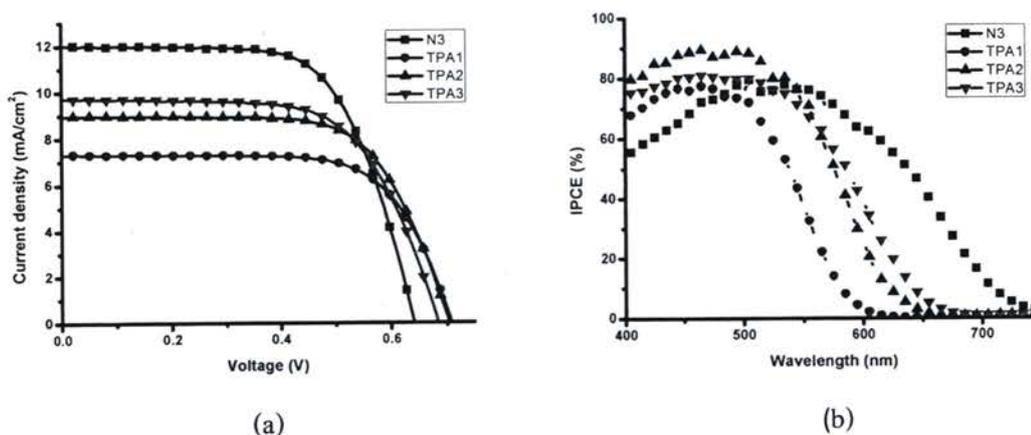
**Figure 4.9** (a) the  $J$ - $V$  characteristics and (b) photocurrent action spectra of DSSCs device based on TPA1-3 sensitizer measured under irradiance of  $100 \text{ mW/cm}^2$  AM 1.5G.
