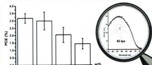
Fig. 5. Power conversion efficiency of DSCs device with difference 400 nm-TiO<sub>2</sub> content (n=3).
