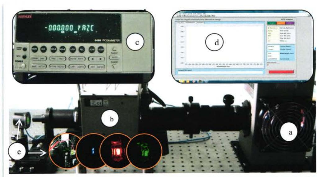
**Figure 3.8** The photograph of IPCE tester. The key components consist of (a) Oriel 96000 solar simulator, (b) Oriel Cornerstone™ 130 1/8 m monochromator, (c) Keithley 6485 picoammeter, (d) front panel of software control and (e) photovoltaic cell.
