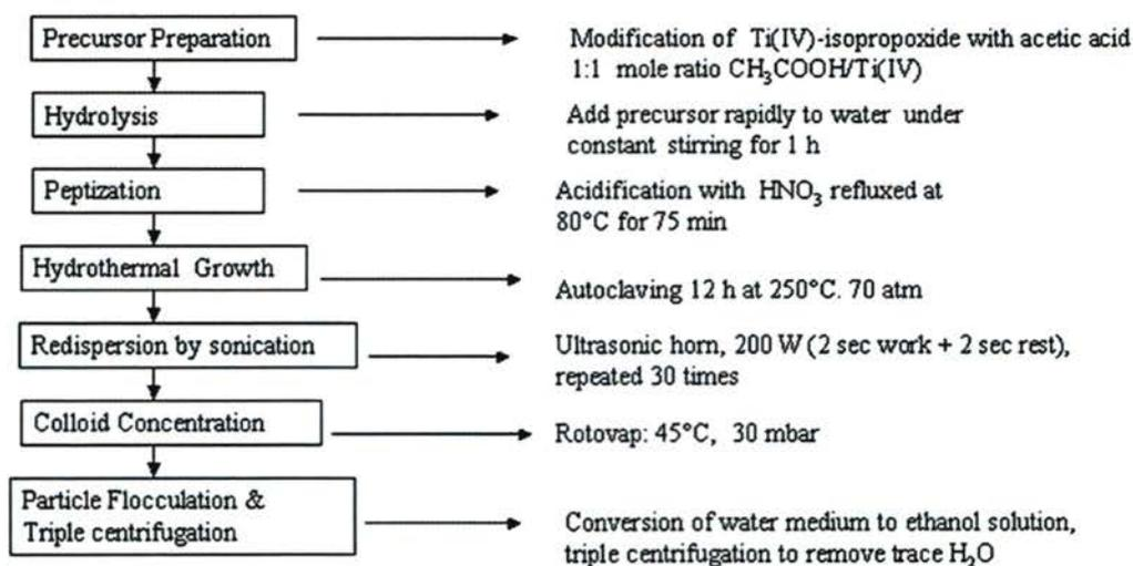
**Figure 2.11** Flow chart of preparation  $\text{TiO}_2$  particle from hydrothermally technique [12].
