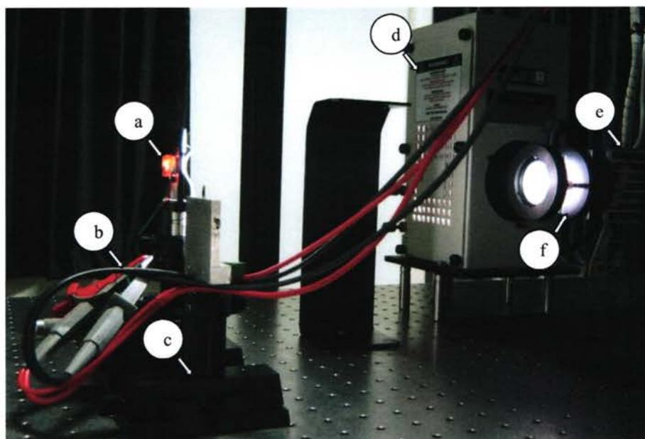
**Figure 3.7** The photograph of *J-V* workstation. The key component of hardware configuration consist of (a) photovoltaic cell, (b) four point probe clamp and solid wire, (c) sample holder with high performance modular ball bearing linear and rotation stages, (d) solar simulator (Newport Oriel 96000), (e) beam turning (Newport 66245) and (f) multiple filter holder and optional filters.
