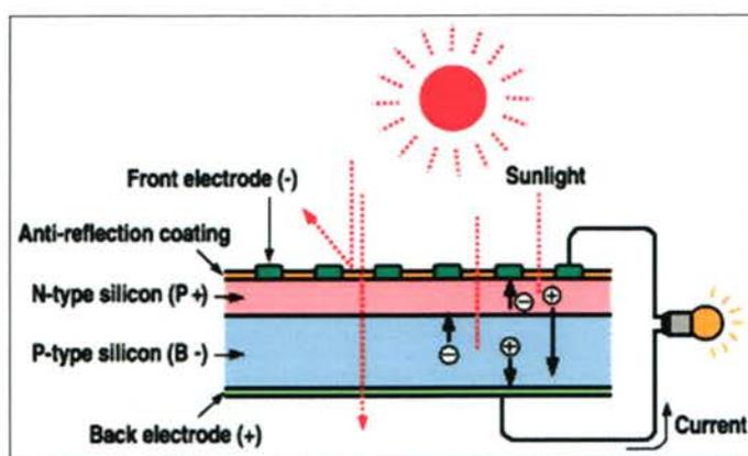
**Figure 1.3** Schematic basic composition of single-junction silicon solar cell [7].
