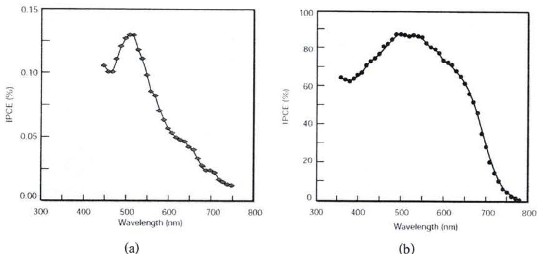
**Figure 2.9** The incident photon to current conversion efficiency of (a) bare TiO<sub>2</sub> electrodes and (b) TiO<sub>2</sub> with sensitized by the surface anchored with ruthenium complex [8].
