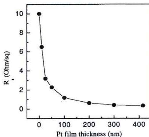
**Figure 2.17** The dependence of sheet resistance of platinized counter electrodes on Platinum film thickness [56].
