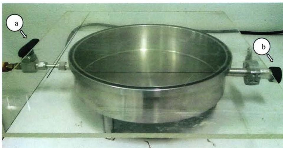
**Figure 3.4** The photograph of the electrolyte filling machine. (a) entrance of vacuum pressure valve and (b) release pressure knob.
