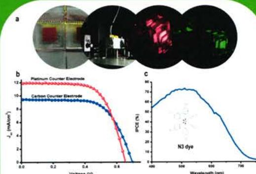
Fig. 4. DSCs device and measurements process (a) I-V curves (b) and IPCE curves (c) of DSC device with platinum and graphite carbon black composites counter electrodes.
