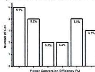
Fig. 5. Histogram depicting reproducibility of DSCs conversion efficiencies. Reported values of 20 DSCs devices produced with same condition.
