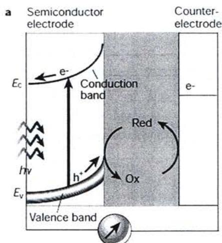
**Figure 2.8** The schematic drawing principle of operation of photo-electrochemical cells based on n-type semiconductors [25].
