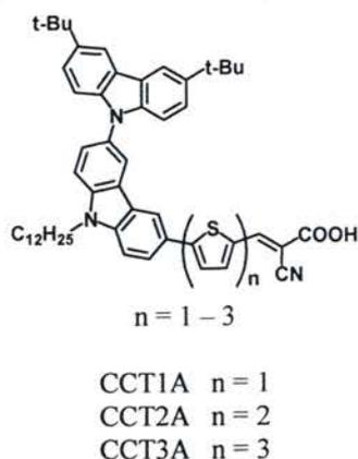
**Figure 4.13** The chemical structure of target dyes (CCT1-3A).
