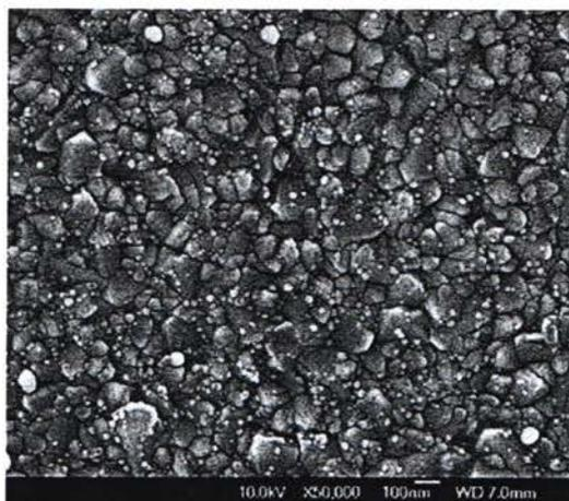
**Figure 2.16** The SEM photograph of platinum counter electrodes surface prepared by electro deposition technique [54].
