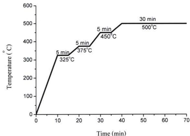
**Figure 3.3** The temperature programs of the working electrode heat treatment.
