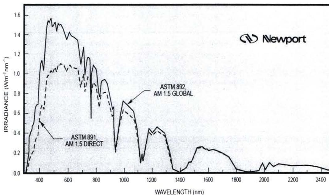
**Figure 2.5** Standard spectra for AM 1.5 [32].
