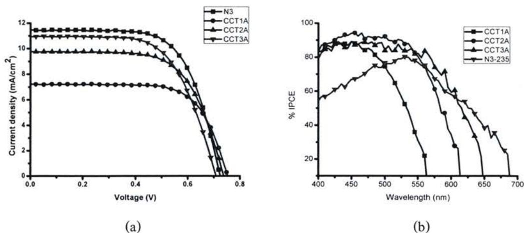
**Figure 4.15** (a) the  $J$ - $V$  characteristics (b) photocurrent action spectra of cells based on CCT1-3A sensitizer measured under irradiance of  $100 \text{ mW/cm}^2$  AM 1.5G.
