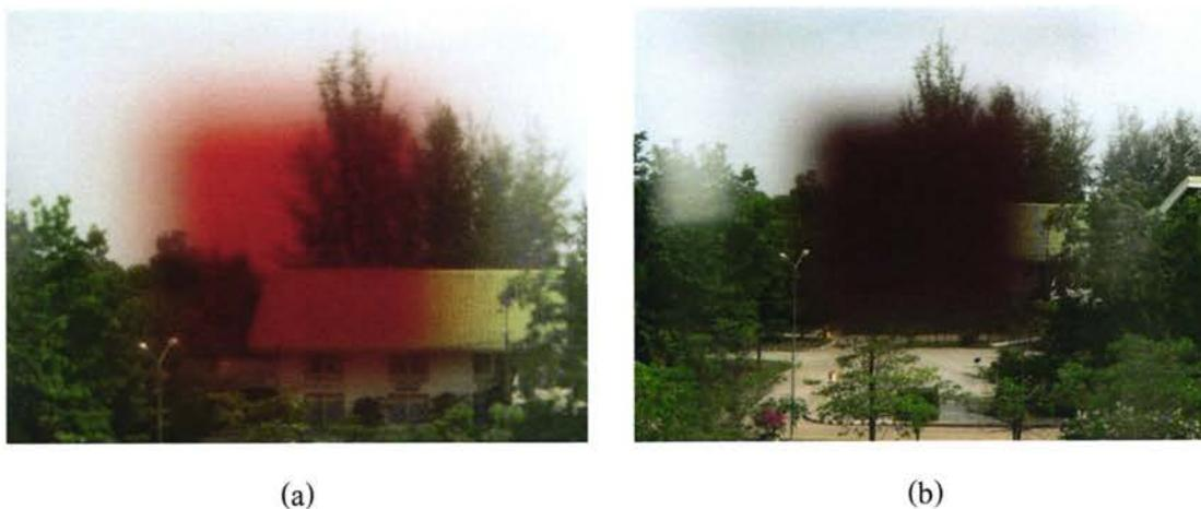
**Figure 4.2** The photograph of monolayer N3 sensitizer on titanium dioxide film coated FTO conducting glass surface, (a) Ti-Nanoxide T20/sp and (b) Ti-Nanoxide R/sp.
