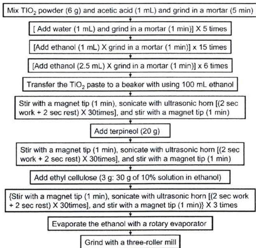
**Figure 2.13** Flow chart of paste preparation from commercially available  $\text{TiO}_2$  powder [40].
