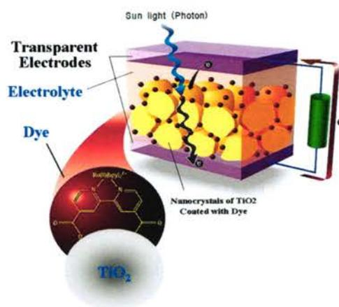
**Figure 1.4** Schematic basic compositions of DSSCs [11].
