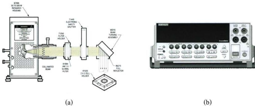
**Figure 3.6** The key equipment of  $J-V$  tester: (a) 96000 Oriel solar simulators and (b) front panel of 2400 Keithley source meter [32].
