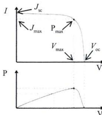
**Figure 2.6** The current-voltage and power-voltage characteristics of photovoltaic cell [34].
