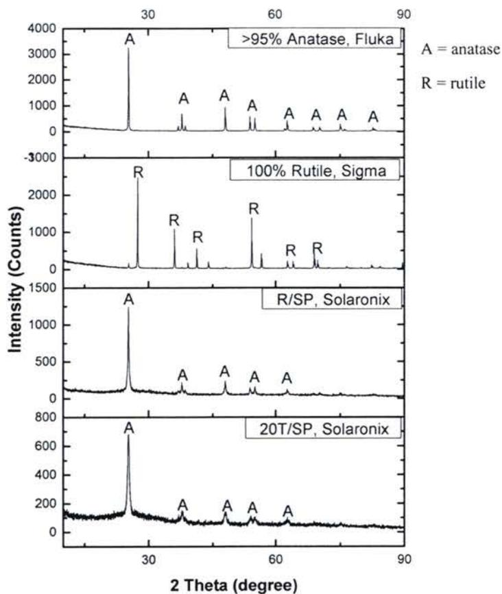
**Figure 4.3** The X-ray diffraction pattern of TiO<sub>2</sub> particle.
