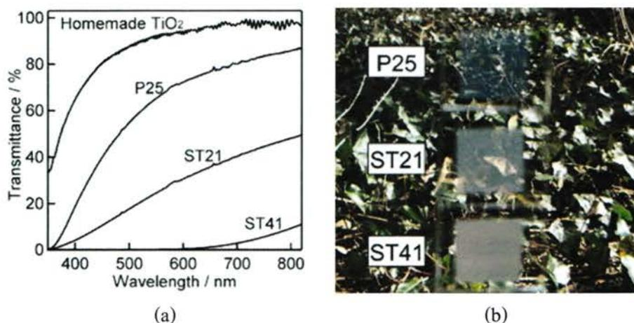
**Figure 2.12** (a) transmittance spectra and (b) photograph of screen-printing paste prepared form commercial available  $\text{TiO}_2$  powder [40].
