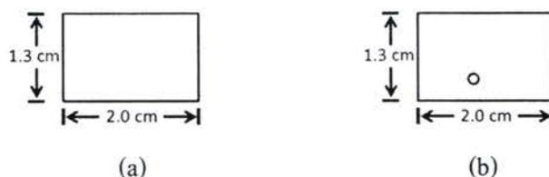
**Figure 3.2** The FTO glass used as (a) working and (b) counter electrode.
