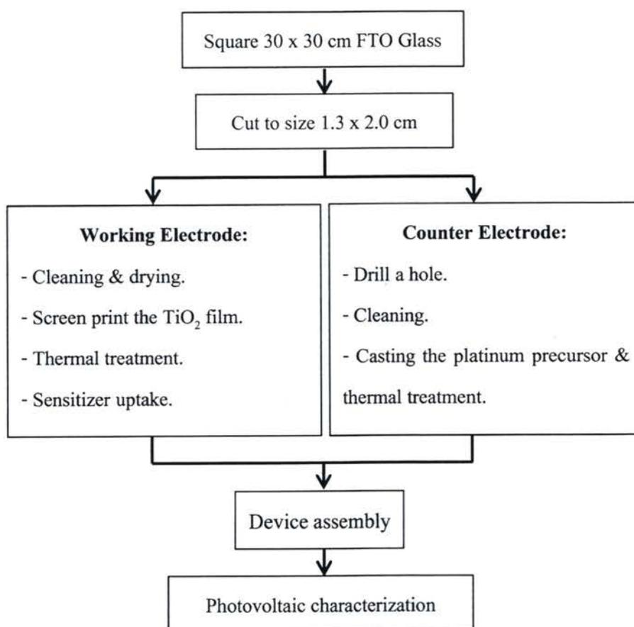
**Figure 3.1** Flow chart of the fabrication and characterization of DSSCs device.
