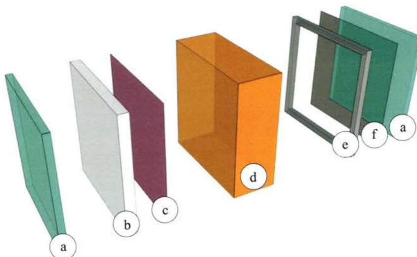
**Figure 2.21** The layout of DSSCs in sandwich type cell design. The DSSCs configurations consist of (a) conductive substrate, (b) Titanium dioxide, (c) sensitizer/dye, (d) electrolyte, (e) sealing gasket and (f) platinum catalyst [71].
