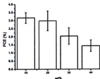
Figure 1. Power conversion efficiency of DSC with difference 400 nm-TiO<sub>2</sub> content.
