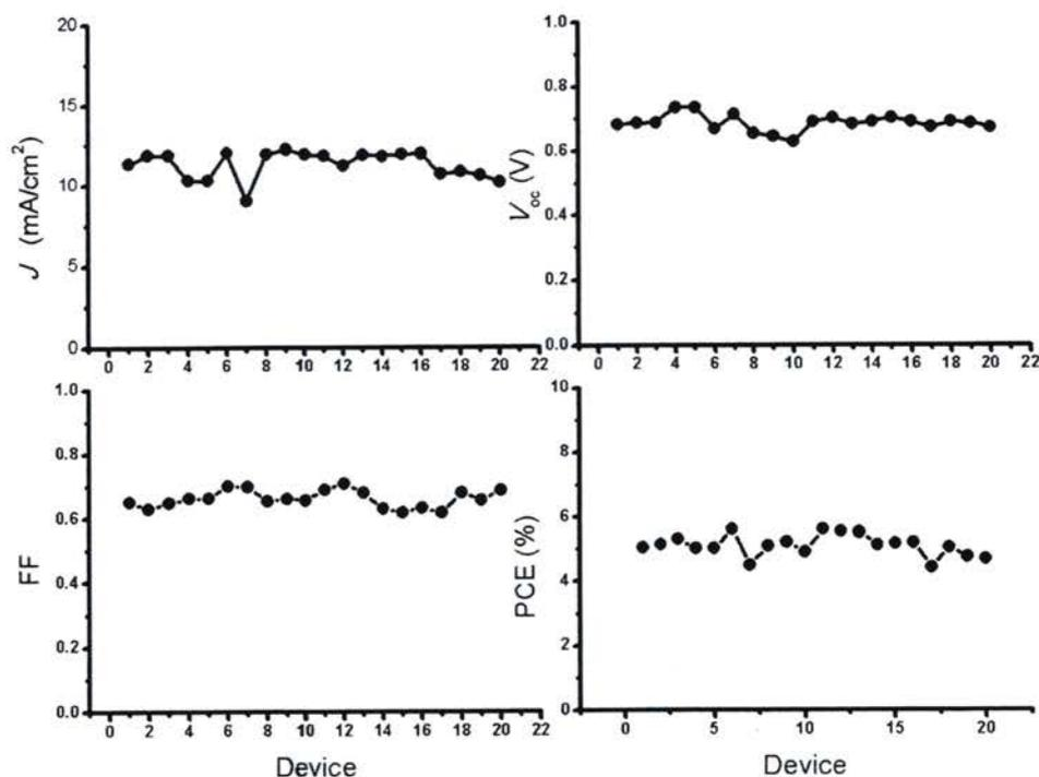
Figure 4.6 The  $J$ - $V$  of DSSC devices in same process.
