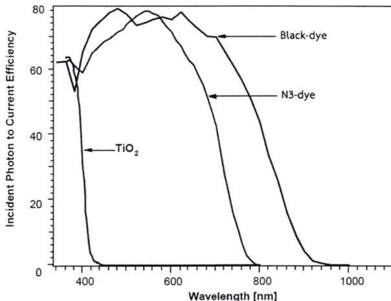
**Figure 2.7** The IPCE spectra obtained with the N3 and the black dye as sensitizer [34].
