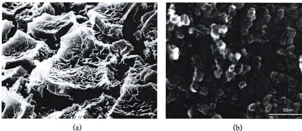
**Figure 2.10** The scanning electron micrograph of a meso-porous anatase  $\text{TiO}_2$  film surface:
