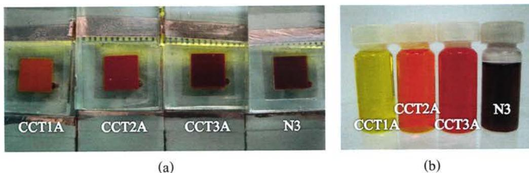
**Figure 4.14** The photograph of (a) DSSC devices and (b) dye solution based on CCT1-3A dye.
