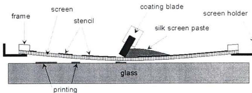
**Figure 2.14** The schematic conceptual of screen printing technique [47].
