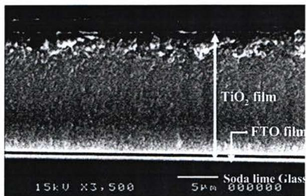
**Figure 4.4** The SEM image of the TiO<sub>2</sub> film coated on the FTO glass.
