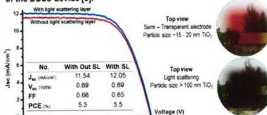
Fig. 4. The I-V curves of DSC device with and with out scattering layer, film thickness 14.68±0.16 μm, base on N3 dye.
