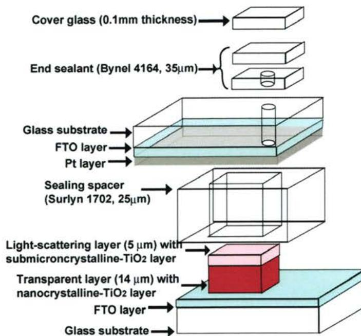
**Figures 2.22** The photograph of layer by layer DSSCs configuration [12].
