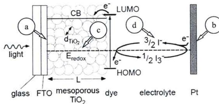
**Figure 2.1** The schematic drawing of the DSSCs key components. The configuration consist of (a) Working electrode (WE): porous  $\text{TiO}_2$  attached to a fluorine doped tin oxide (FTO), (b) Counter electrode (CE): platinum nano particle attached to a fluorine doped tin oxide (FTO), (c) Light absorbing layer: adsorbed sensitizing dye/ chromophore and (d) Redox system: liquid electrolyte containing the iodide/tri-iodide ( $\text{I}^-/\text{I}_3^-$ ) [23].
