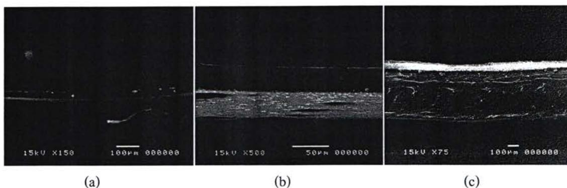
**Figure 4.1** The cross section SEM photograph of sealant materials. (a) Surllyn<sup>®</sup> 30, (b) Para film M and (c) EVA film.
