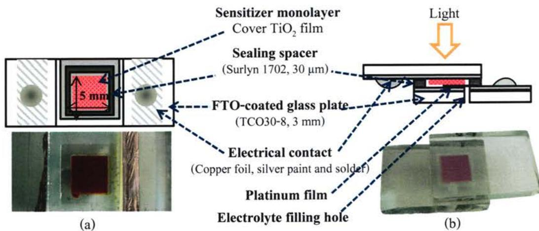
**Figure 3.5** The photograph and schematic drawings cross section of the DSSCs test cell.
