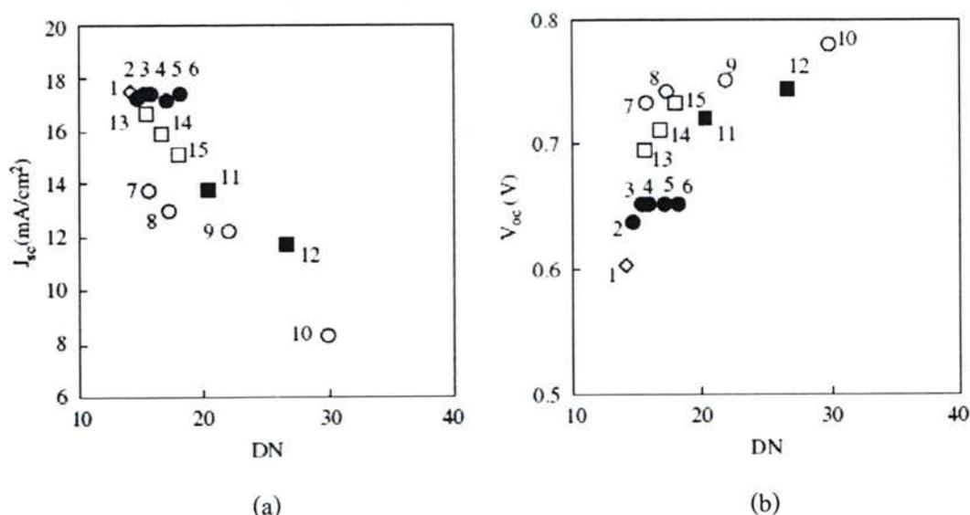
**Figure 2.18** Dependence of (a)  $J_{sc}$  and (b)  $V_{oc}$  of DSSCs on the donor number of solvents [59].
