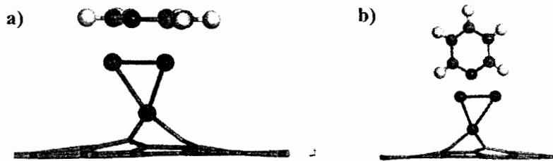
**Fig. 5.** Side view of VOC initial configurations (a) parallel and (b) perpendicular to the TM tetramer cluster of the TM-doped SDG surface.
