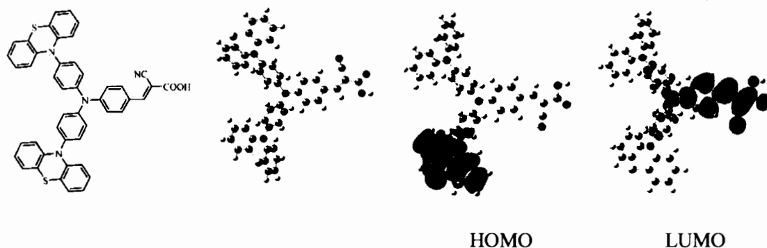
Figure 2.5 Molecular structures, optimized geometries, and molecular orbital distribution of PTZ-1
