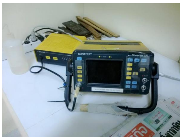
Figure A.7 Ultrasonic flaw detector (SONATEST: SITESCAN 230)
