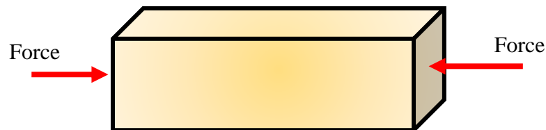
Figure 2.13 Longitudinal modulus in materials
