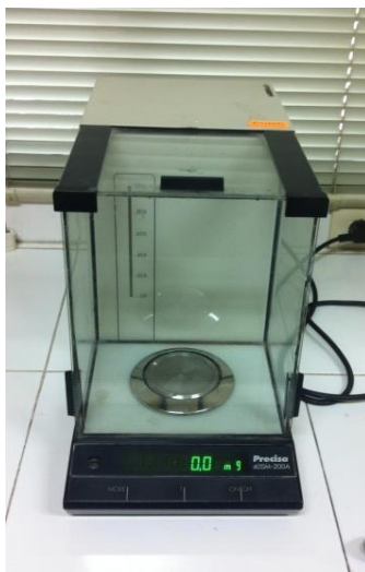
Figure A.1 Electronic balance (Precisa d05M-200A) having an accuracy of 0.0001 g
