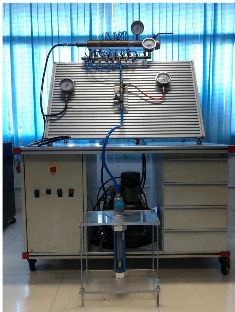
**Figure 3.7 The experimental SSE gas/gas ejector system**
