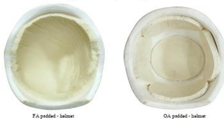
(b) Layout of rubber sponge pads for FA and OA helmets
