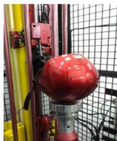
Figs. 4. Drop test setting up
